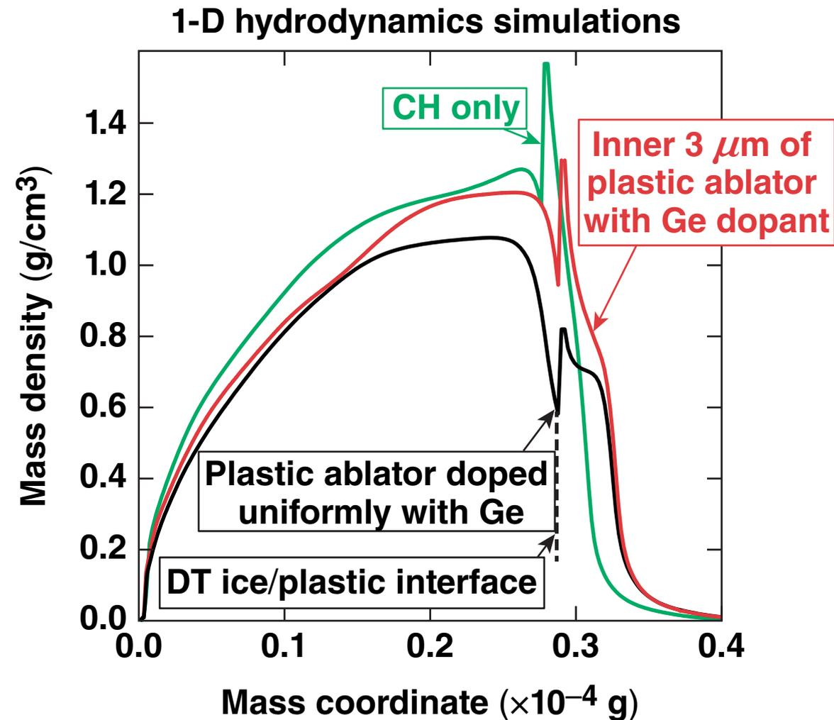
The DT ice/CH interface is not stable for the plastic ablator doped uniformly with Ge.
