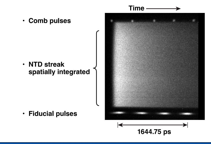
Comb and fiducial pulses are used to compensate for streak-camera distortions.
