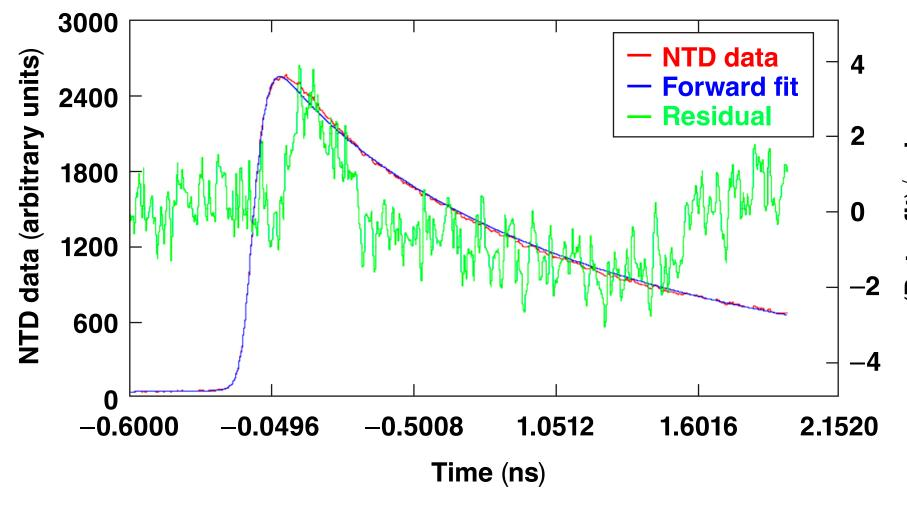
NTD model compares well with the measured data;  $0.5 < \chi^2_{DoF} < 2.0$ .
