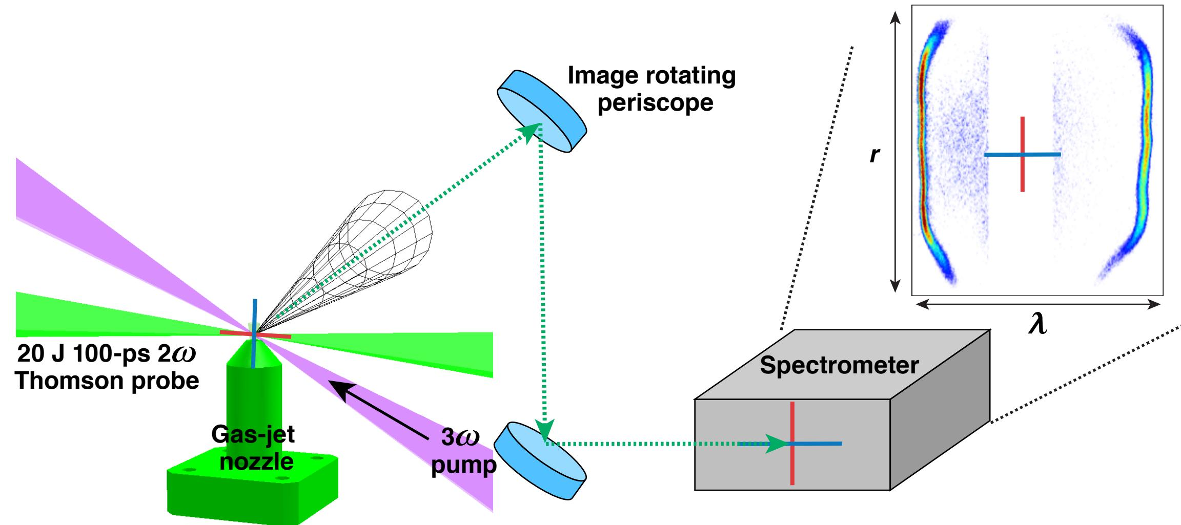
$2\omega$  imaged Thomson scattering was used to measure the spatial density and temperature profile of the target plasma
