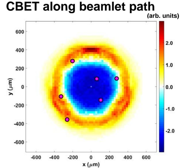
Beamlet spot intensities will be used to verify (CBET) mitigation with the new TOP9 variable wavelength beam.<sup>1</sup>
