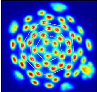
Beams are grouped according to their radial position, e.g., Beam Group 1 is the innermost five spots
