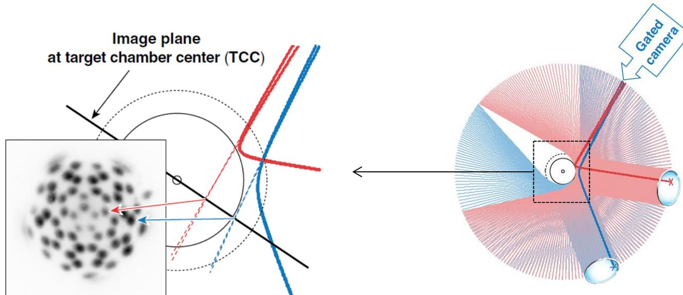
**The radial position of each beamlet spot depends only the incident beam direction (fixed for OMEGA geometry) and on refraction through the density profile**
