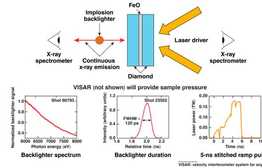
Using the ramp-compression platform, FeO will be studied at high pressures and temperatures
