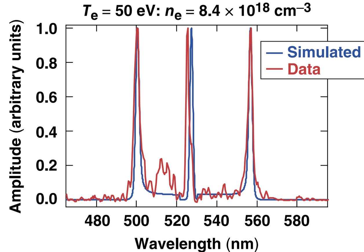
Keeping the electron density constant, the Thomson spectra were fit for all earlier times by changing the plasma temperature.
