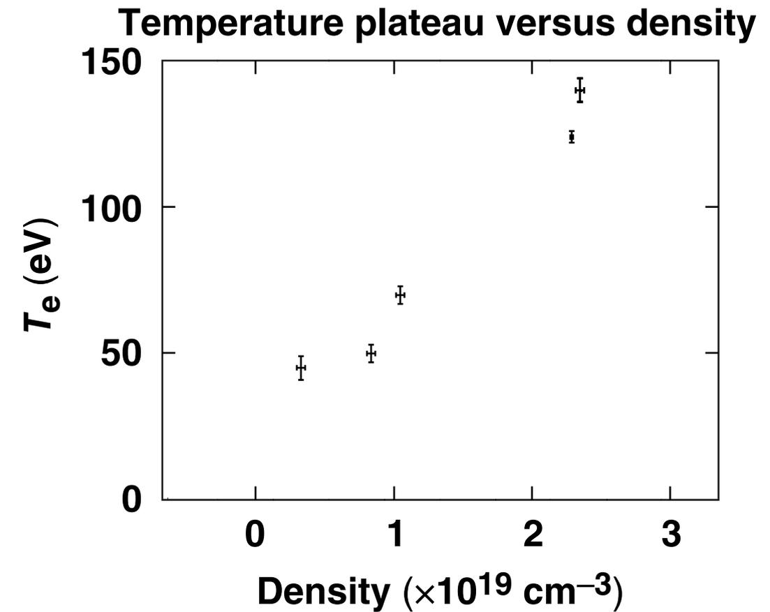
As opposed to a free parameter, the temperature in a Raman amplifier is determined by the plasma density for a fixed pump intensity.
