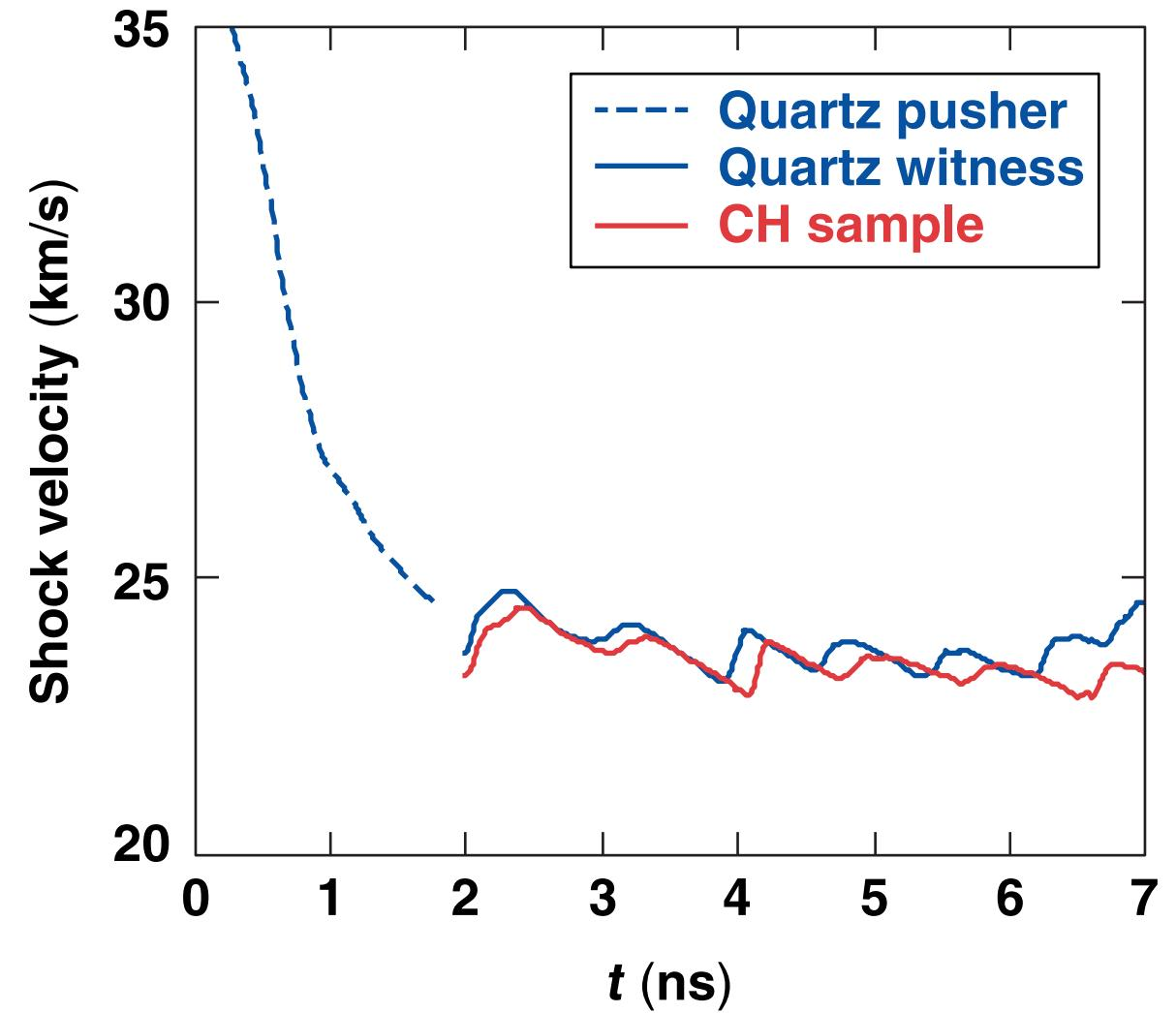
The difference in arrival times is used to infer sound speed.
