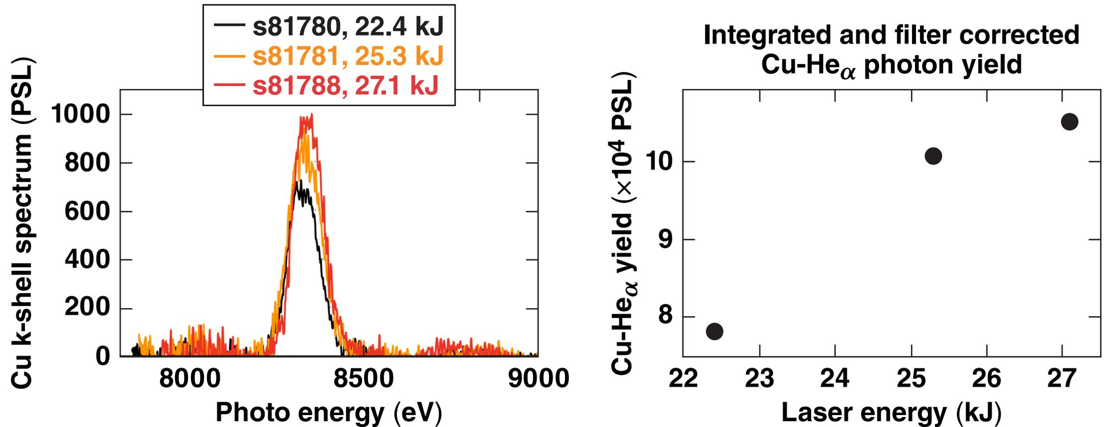
The observation of the hot-ionic line and the absence of the cold  $\text{Cu-K}_\alpha$  line indicates the creation of hot dense matter caused by shock heating of the Cu particle in the center.
