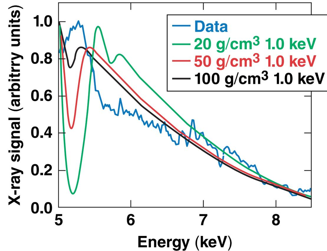
A temperature of  $\sim 1 \text{ keV}$  and a mass density of  $100 \text{ g/cm}^3$  indicates that a pressure of Gbar has been reached inside the titanium sample.
