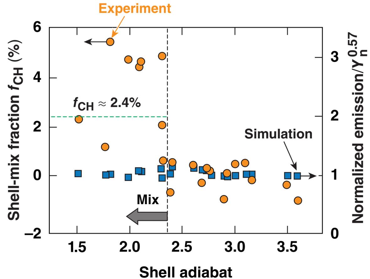
X-ray spectroscopy experiments were conducted on OMEGA to diagnose the hot-spot mix.
