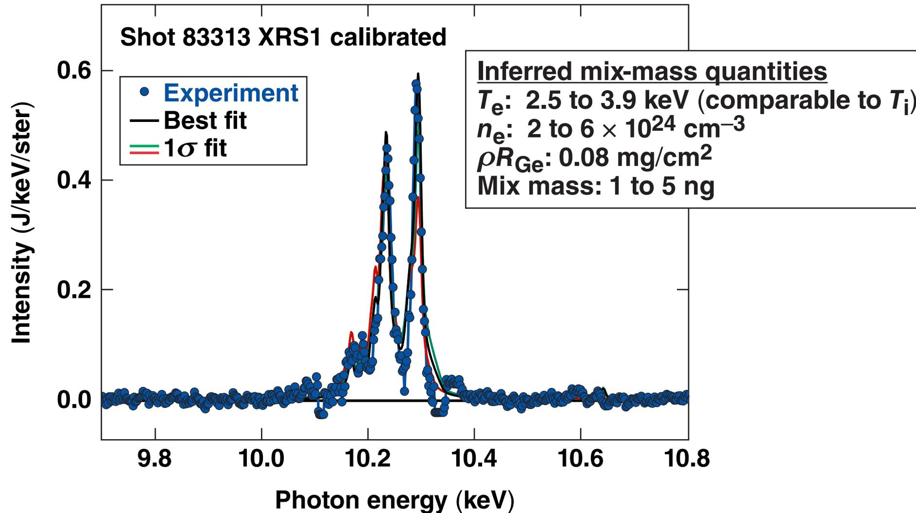
The brightness of the Ge K-shell emission depends on  $n_e$ ,  $T_e$ , and  $\rho R_{Ge}$ .
