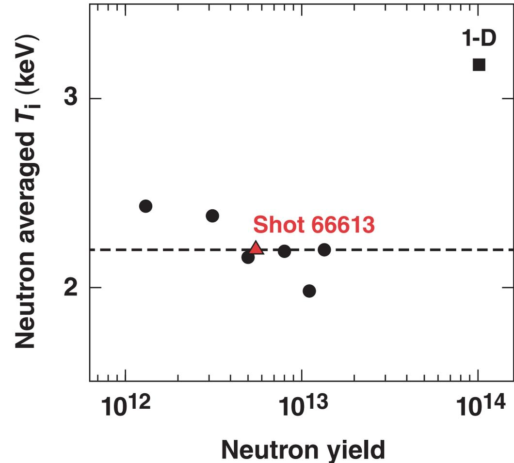
**The mixing of ablator mass into the hot spot reduces target performance.**
