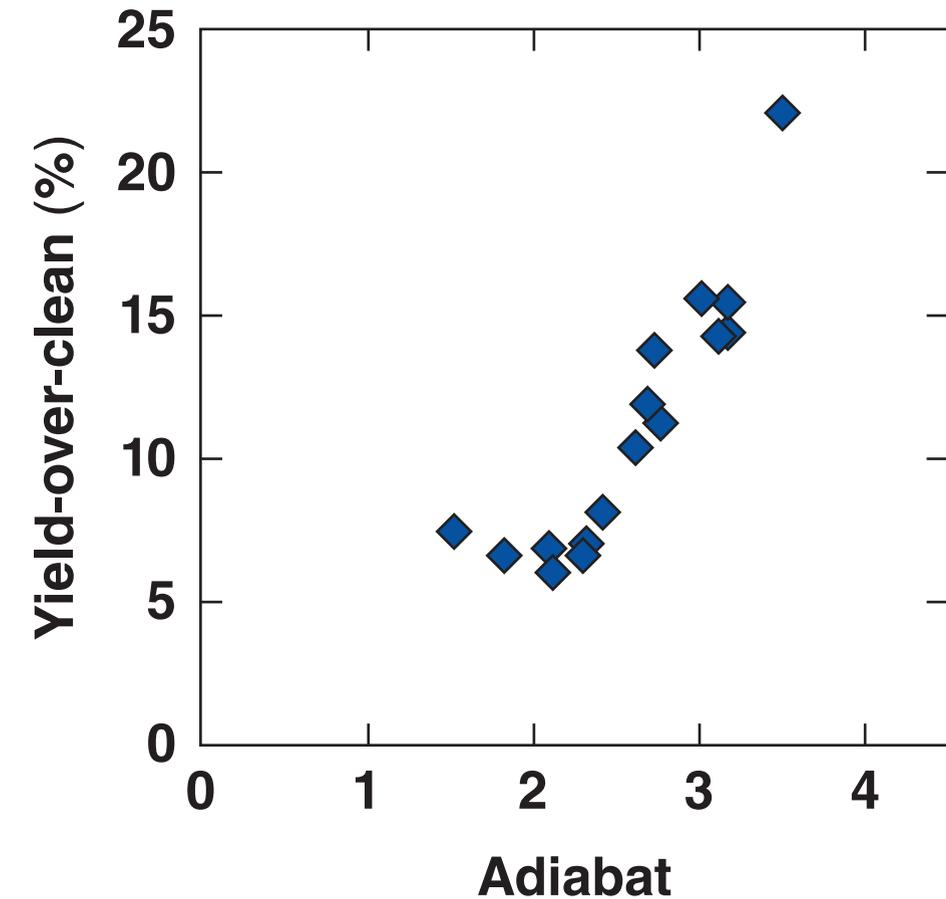
The 2-D simulations predict a degradation in target performance caused by mixing the ablator into the hot spot.
