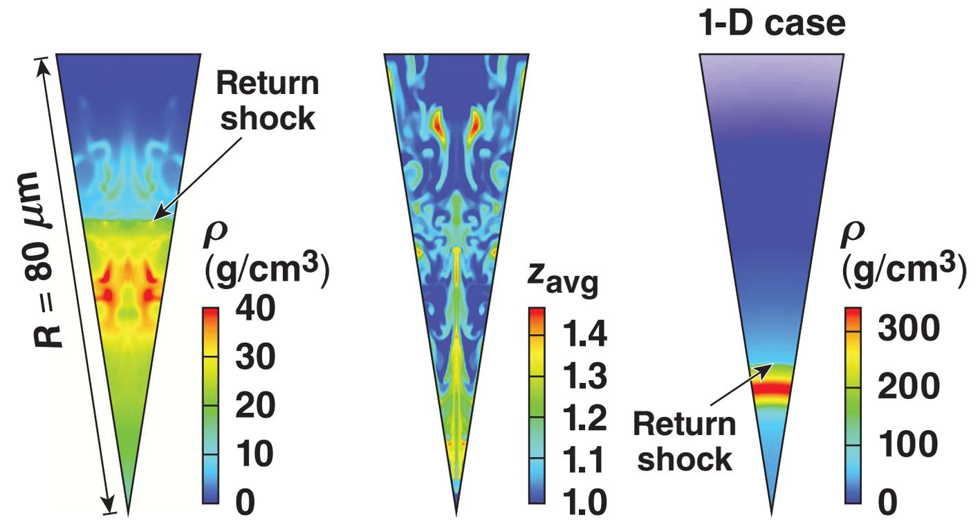
The ablation-front instability causes the ablator material to be mixed into the compressed fuel and hot spot.
