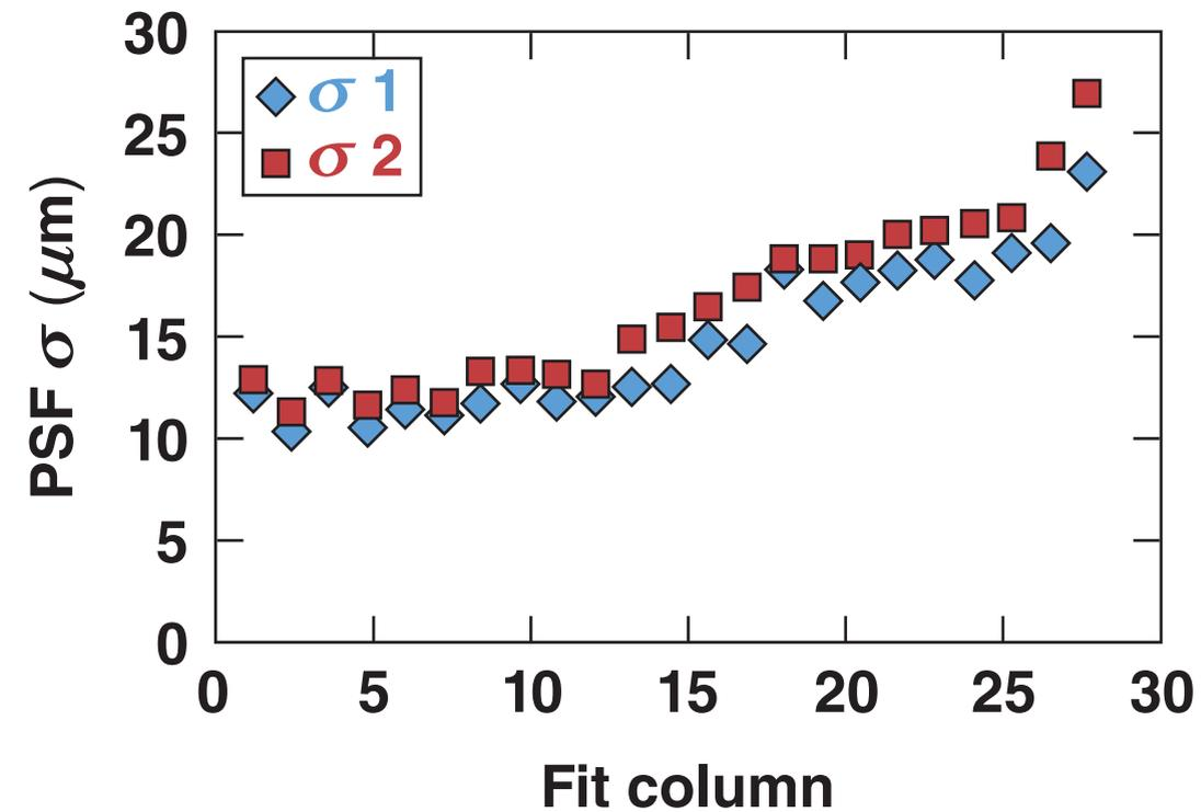
Late-time data show that the Ta wires expand because of x-ray absorption.
