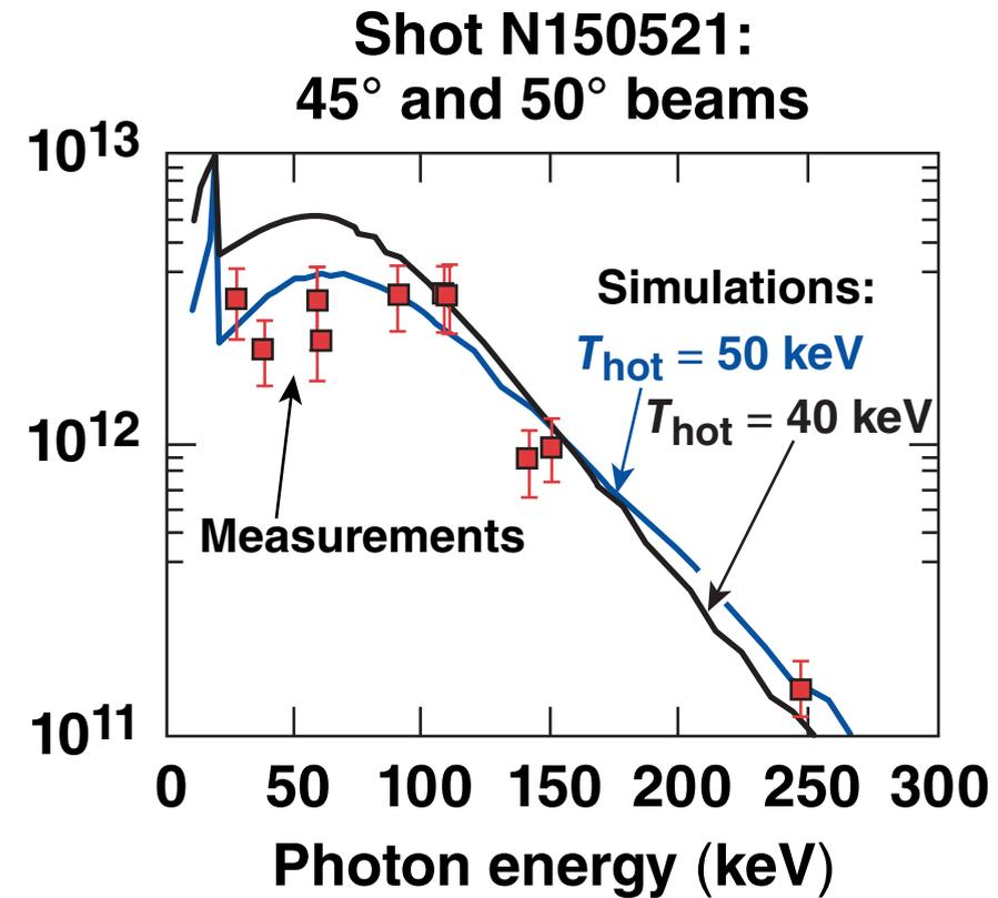
Time-integrated hard x-ray spectra indicate  $T_{\text{hot}} = 40$  to 50 keV, consistent with TPD.
