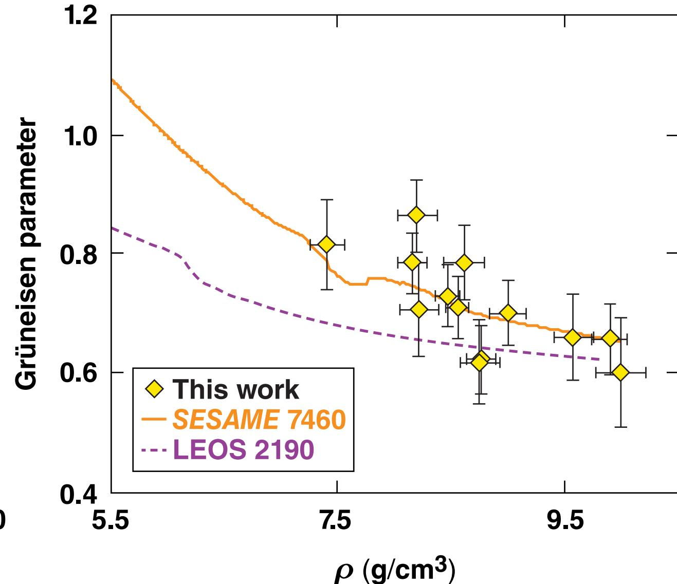
**The sound speed and Grüneisen parameter in polystyrene (CH) and periclase (MgO) were measured from the propagation of known acoustic disturbances**
