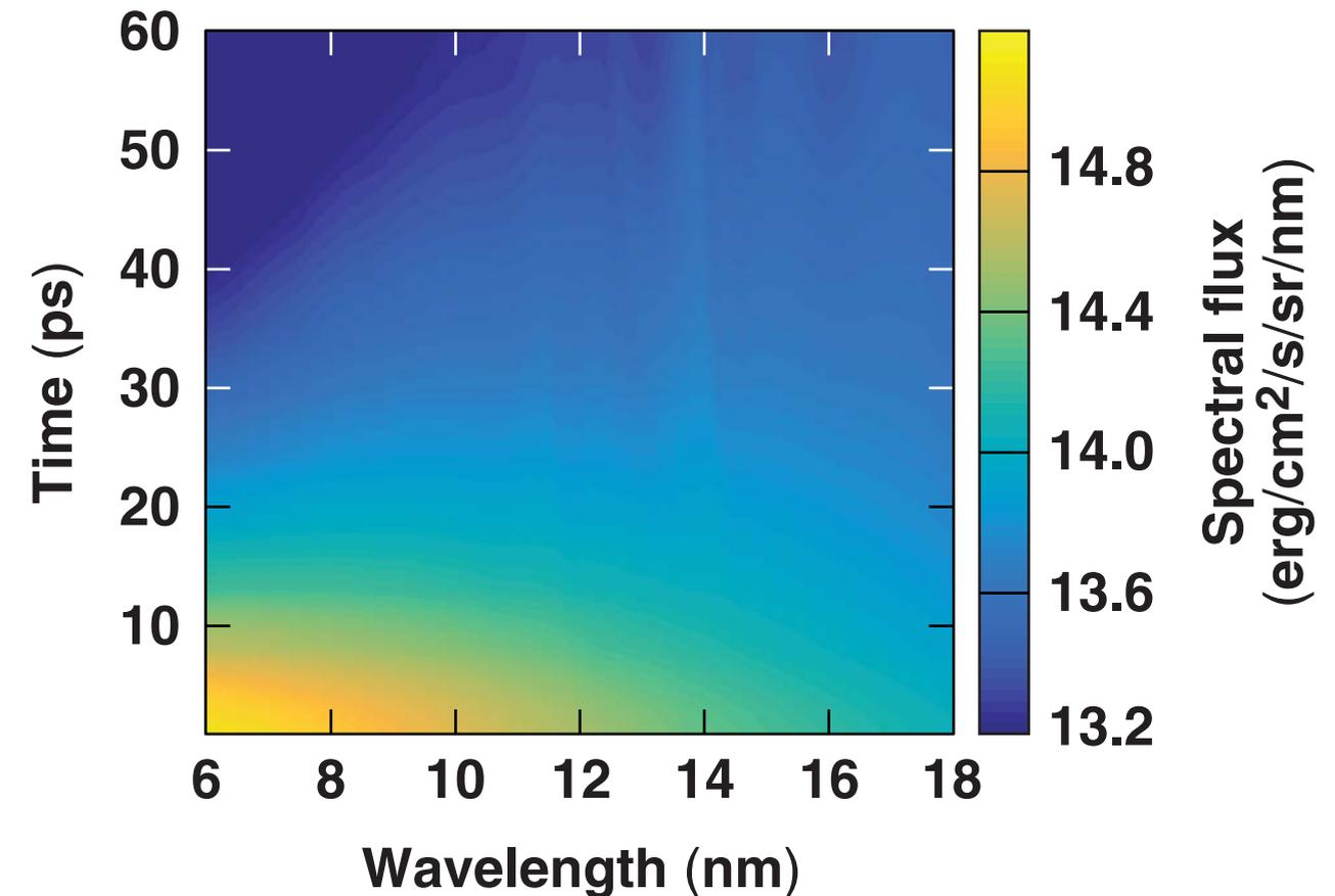
The temperature of the target can be inferred from the local slope of the continuum emission.
