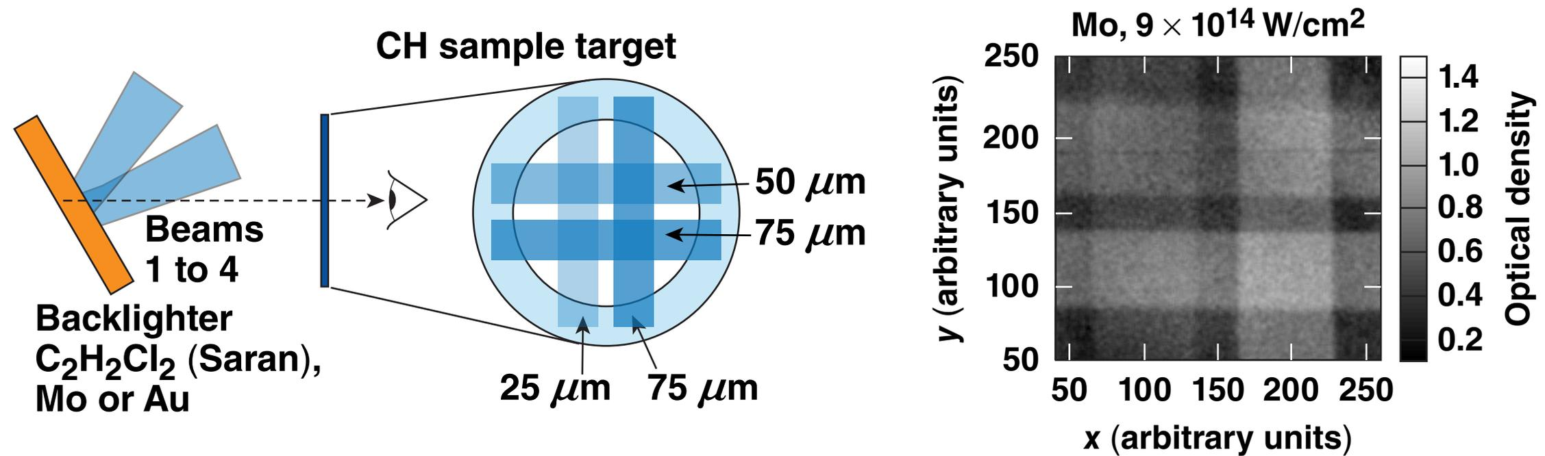
Best brightness and contrast were achieved for a Mo L-shell backlighter at  $9 \times 10^{14} \text{ W/cm}^2$ ,  $\sim 4\times$  brighter than Saran.
