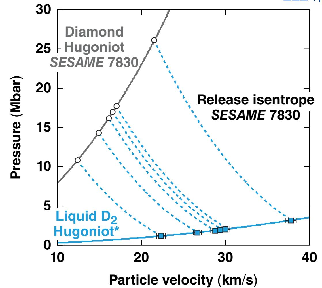
The SC diamond release into liquid D<sub>2</sub> is accurately modeled using SESAME 7830.
