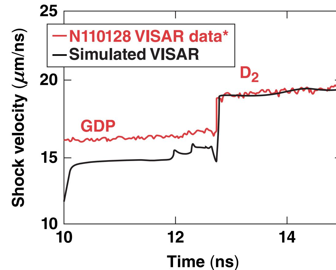
The glow-discharge polymer (GDP) equation-of-state model was corrected using release data into liquid D<sub>2</sub>.\*\*
