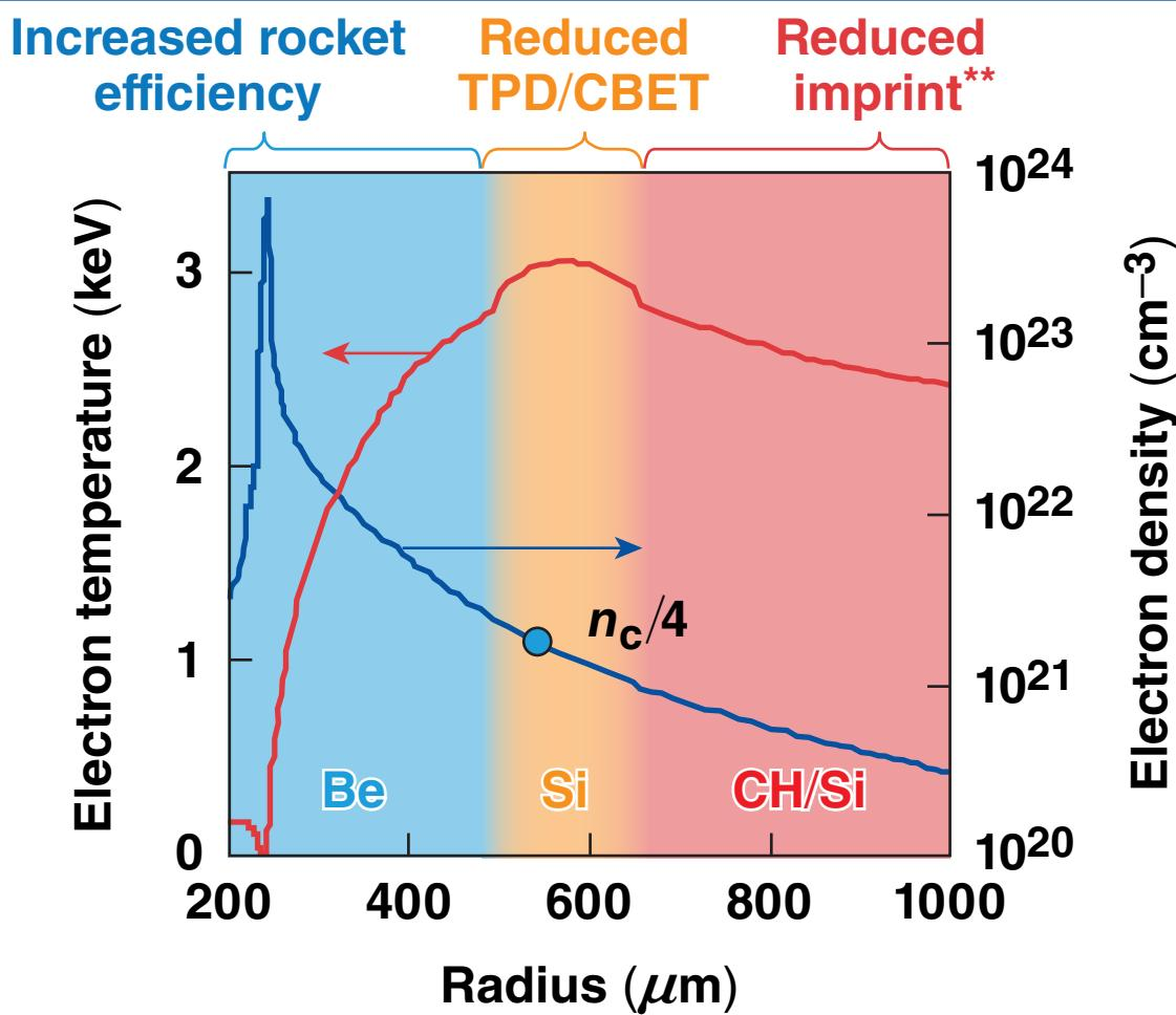
The layer thicknesses are optimized to have increased laser absorption at  $n_c/4$  (Si higher  $T_e$ ) and increased ablation in Be (higher  $A/Z$ ).
