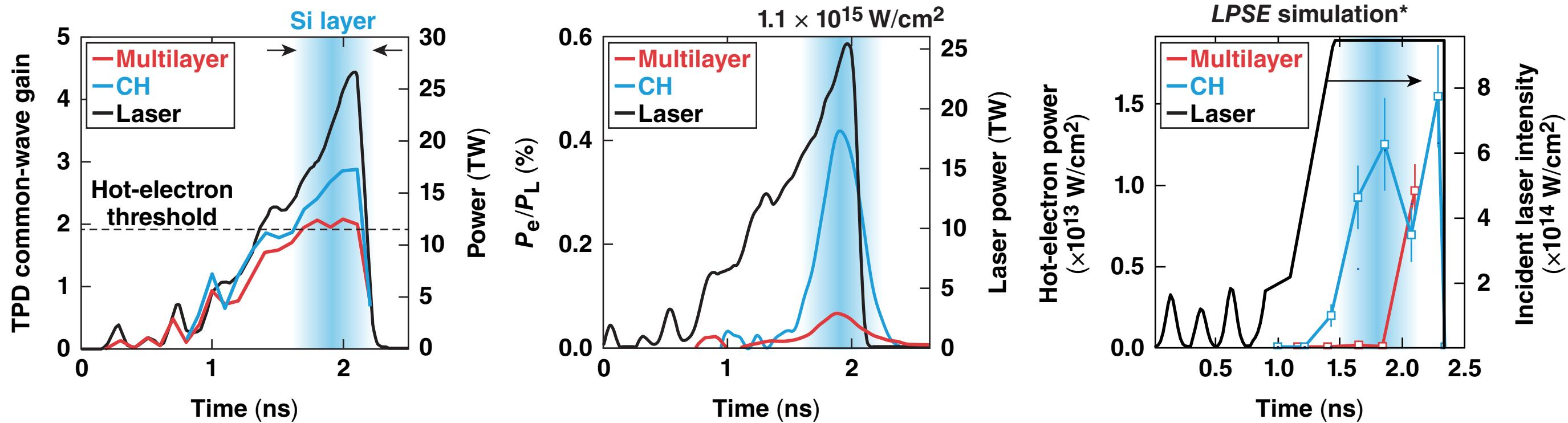
The hot-electron fraction is reduced by a factor of 8 in multilayer targets compared with CH.
