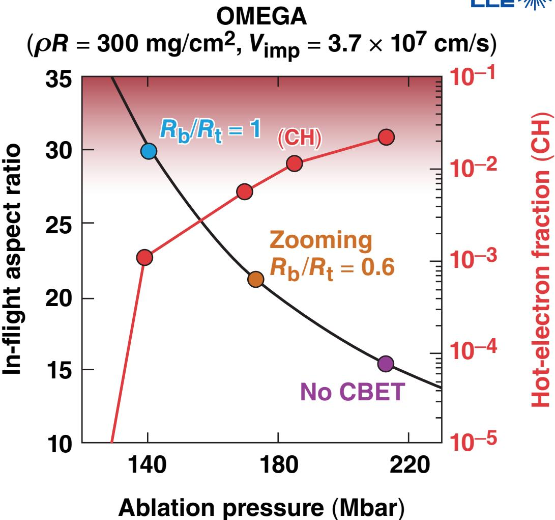
Current cryo experiments show no evidence of hot-electron preheat, but simulations suggest a factor-of-2 increase will degrade the areal density.
