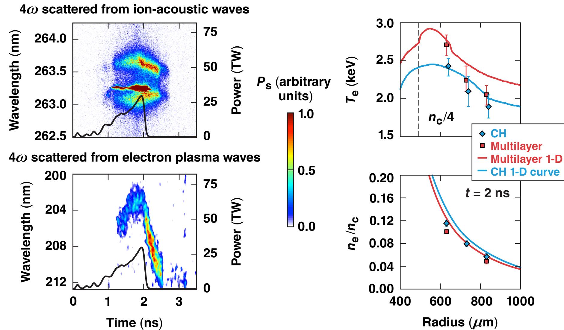
Multilayer ablators increase the electron temperature around quarter critical by ~15%.
