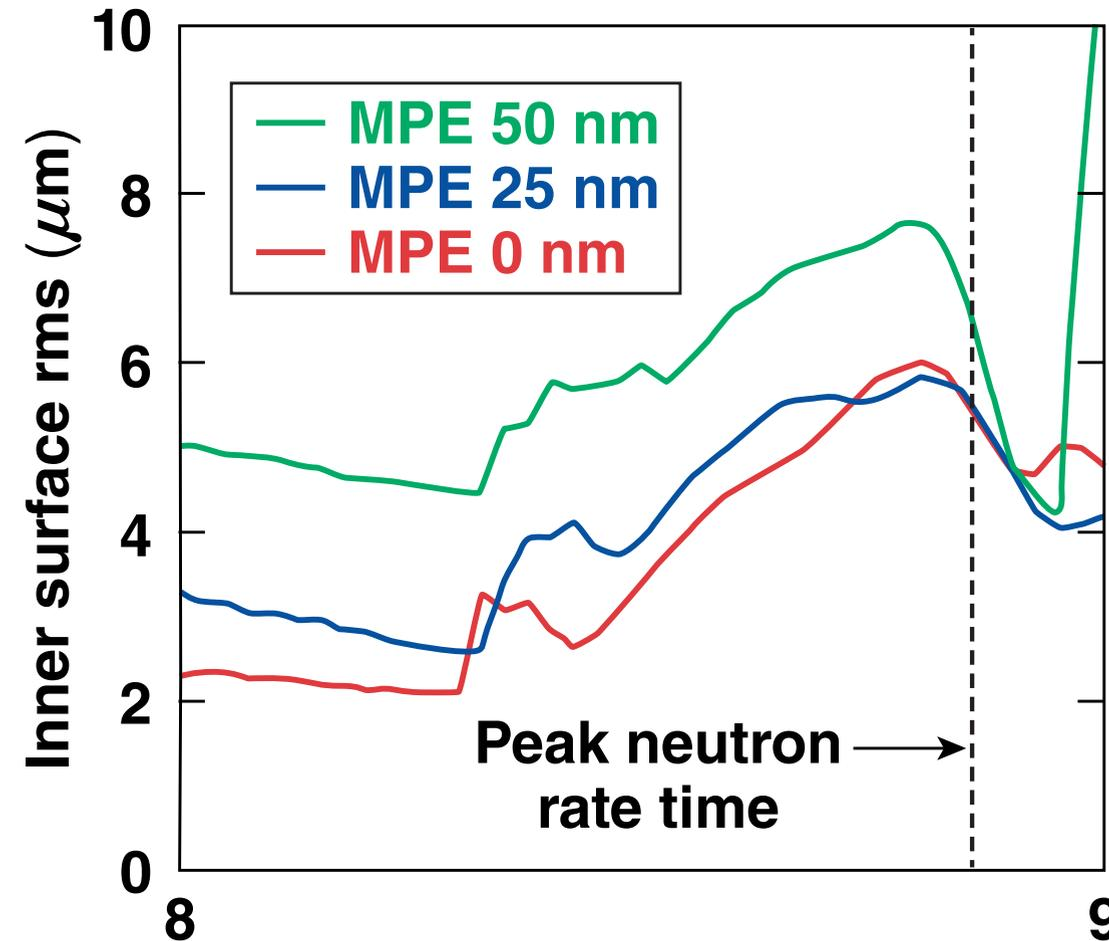
Reducing iDPP MPE to below 25 nm gives a diminishing return for minimizing the inner surface rms.
