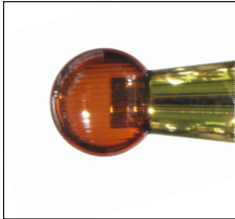
Cone-in-shell CH target
