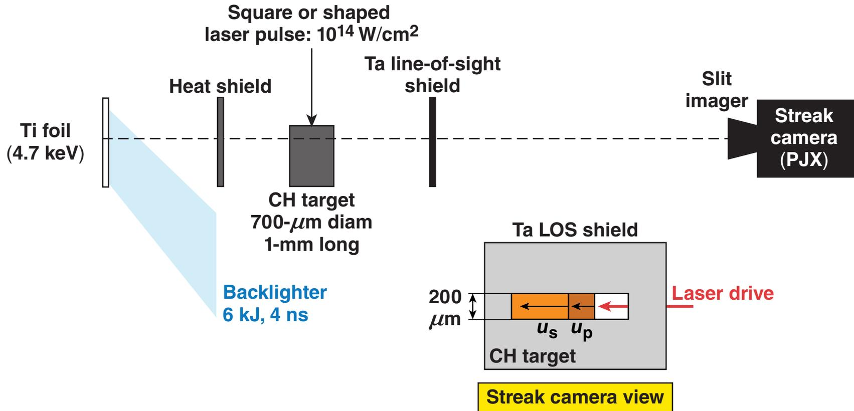
The open-drive geometry allows for radiographic access to the ablatively driven piston.
