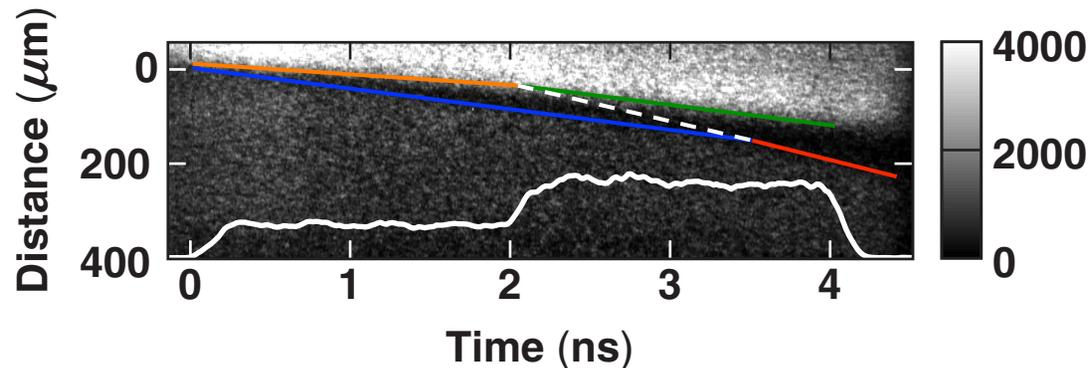
— Piston 1 — Piston 2 — Shock — Strengthened shock
