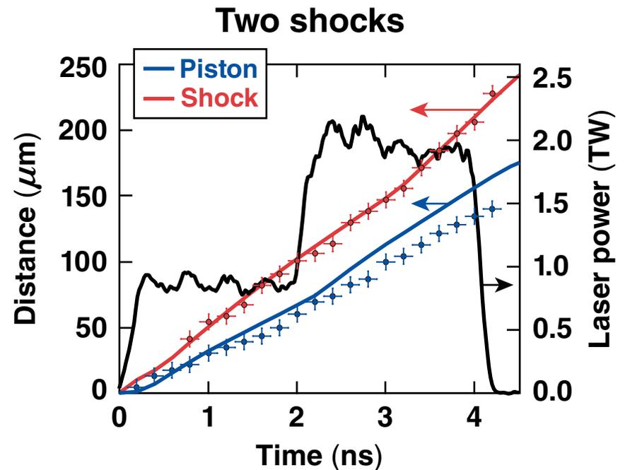
The *DRACO*-predicted piston velocities are higher than the experimental measurements.
