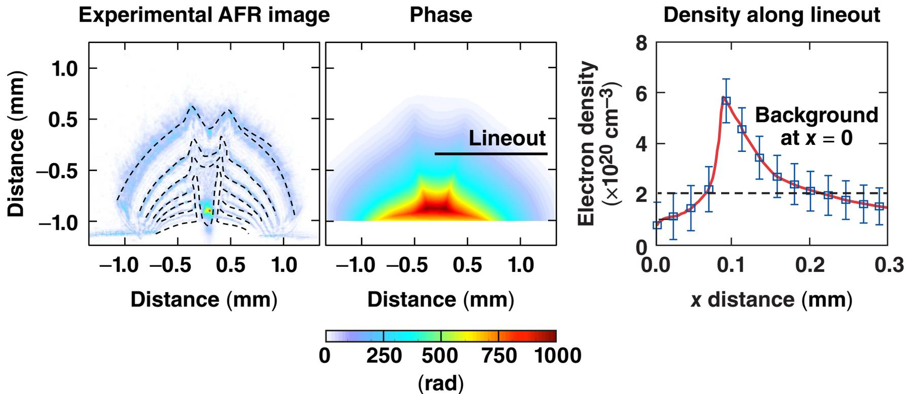
The density in the channel is reduced to  $(1 \pm 0.75) \times 10^{20} \text{ cm}^{-3}$ .
