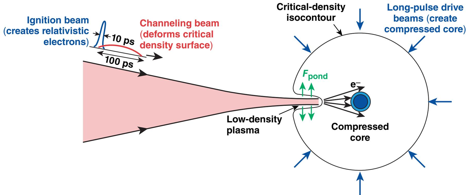
The channeling beam evacuates the coronal plasma ahead of a second laser pulse used to heat the core of an imploded target.
