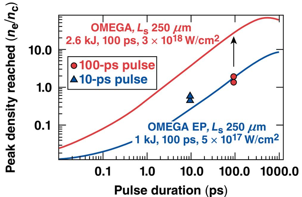
This model suggests that a full-energy (2.6-kJ, 100-ps,  $3 \times 10^{18} \text{ W/cm}^2$ ) OMEGA EP beam may reach up to  $25 n_c$  in a shorter-scale-length OMEGA implosion ( $L_s \sim 100 \mu\text{m}$ ).
