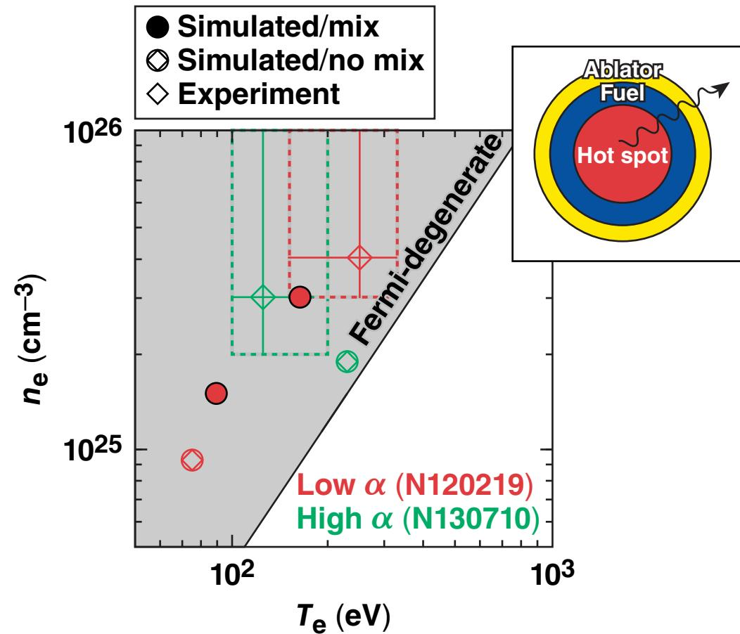
Hydrodynamic mixing of the ablator and fuel layers increases the inferred  $T_e$  and  $n_e$ , indicating there is more mix for the low-adiabat implosion.
