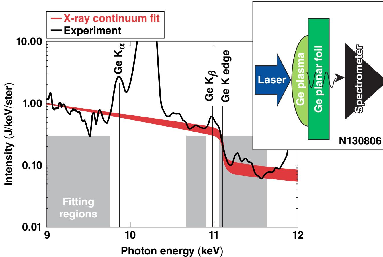
$\rho R_{\text{Ge}} = 8.3 \text{ } (-2.8, +0.1) \text{ mg/cm}^2$  is inferred from this calibration shot using the cold opacity.\*
