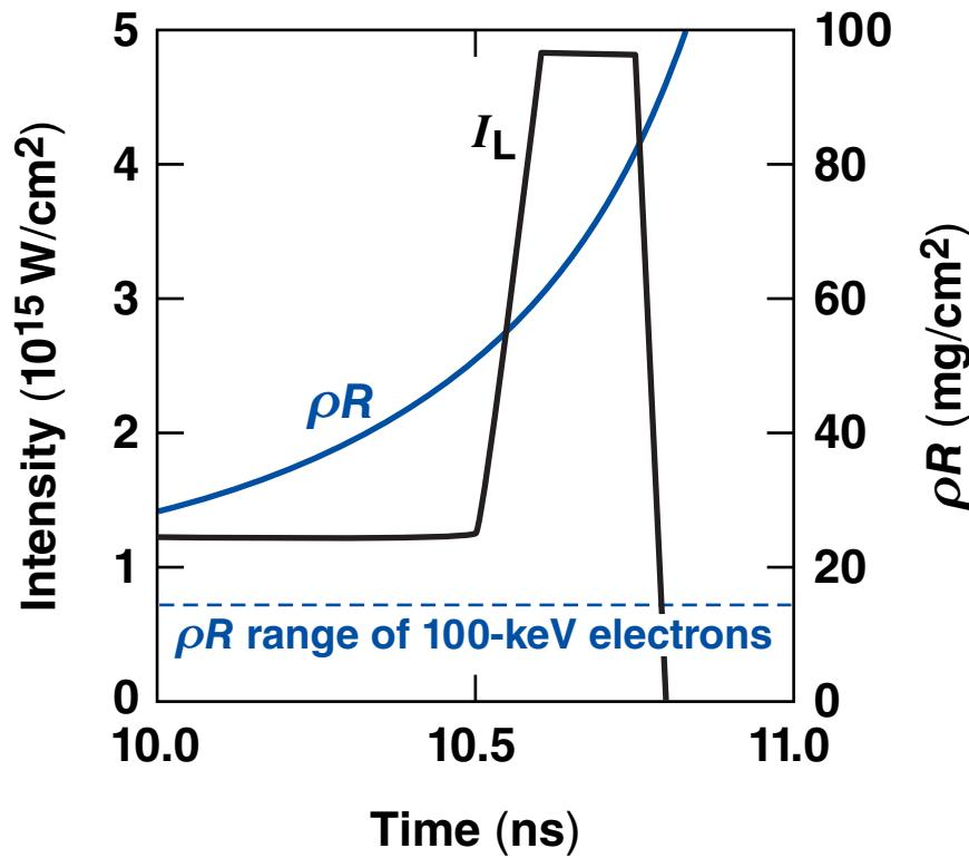
For low-enough energy, hot electrons are stopped in a narrow outer layer of the imploding shell.
