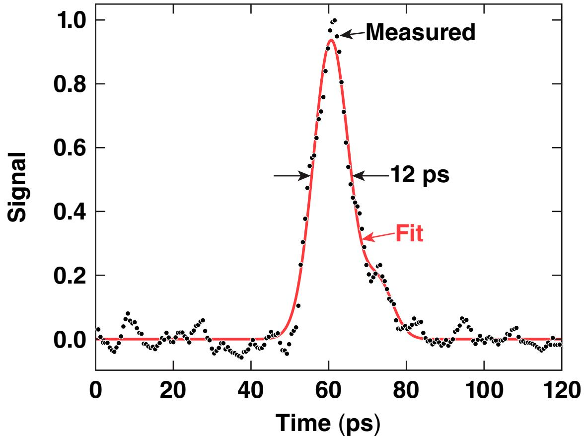
Time-resolved  $K_{\alpha}$  x-ray emission from a Cu foil target irradiated with a  $\sim 1$  kJ, 10-ps pulse.\*
