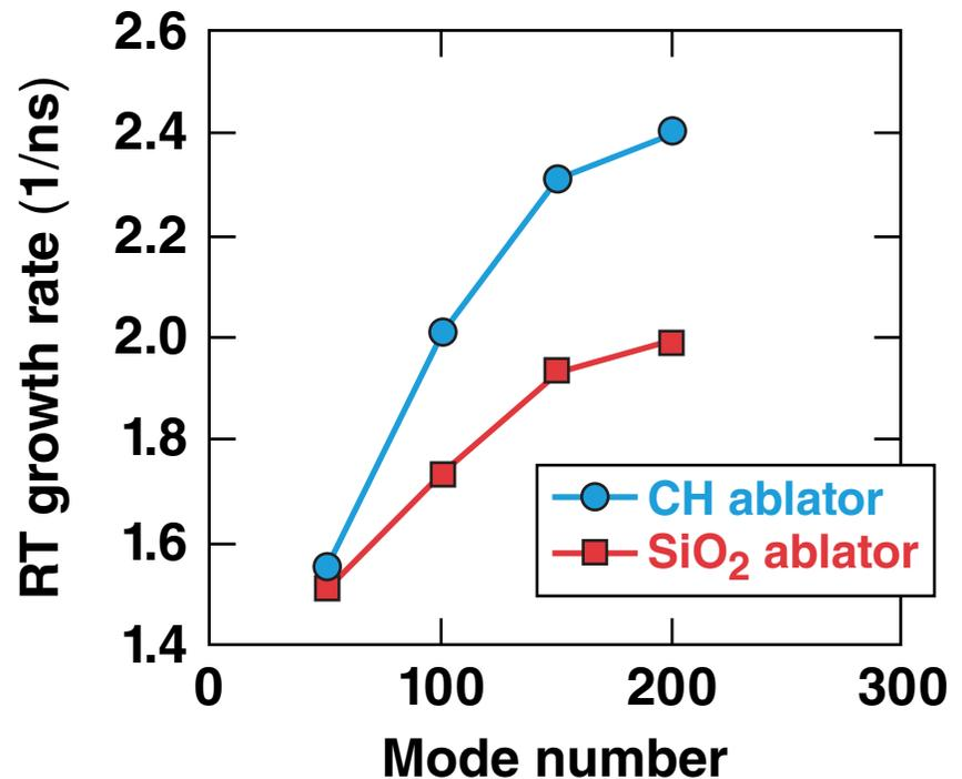
Using graded doping of plastic layers reduces the RT growth in a double-ablation-front structure.
