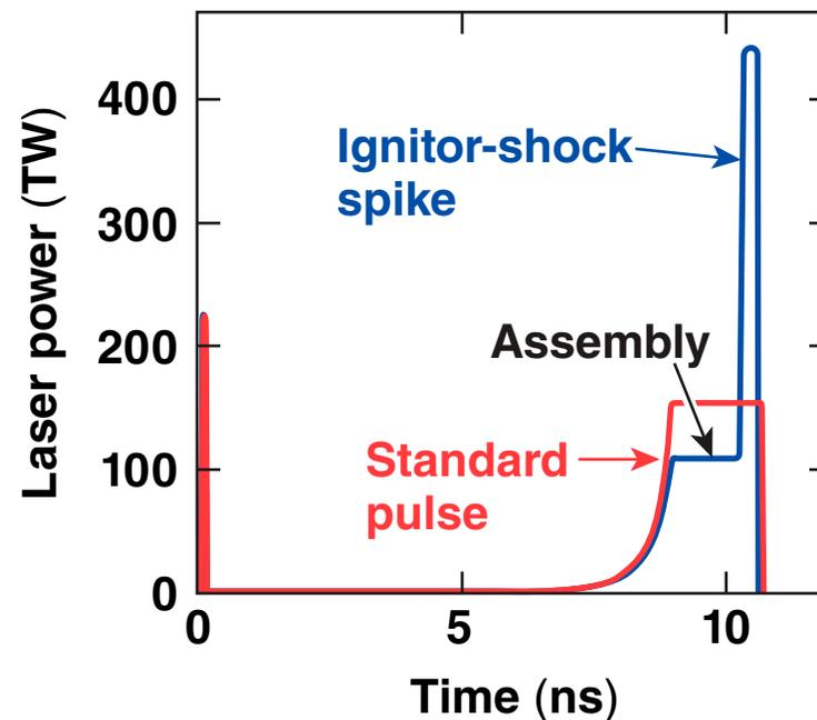
**The high-intensity spike needs to generate ~300-Mbar of ablation pressure.\*\***
