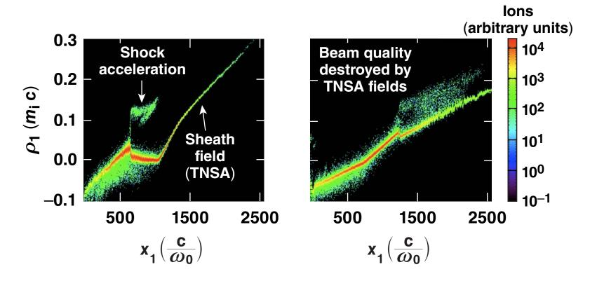
Sheath fields that exist at the sharp plasma vacuum boundary can smear the energy spread of accelerated ions.
