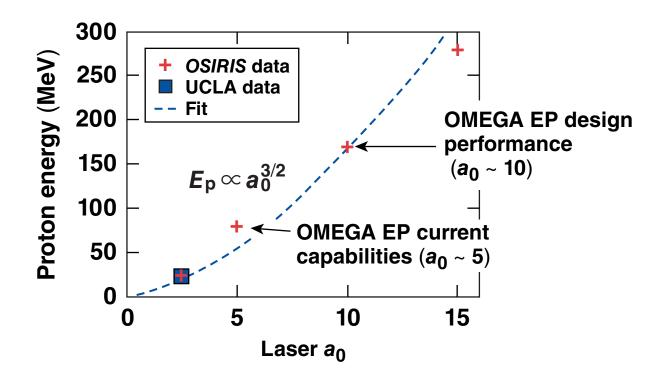
Scaling the SWA mechanism to the 1- $\mu$ m OMEGA EP Laser System allows for the production of narrow energy spread ion beams in the 100- to 200-MeV/amu range.
