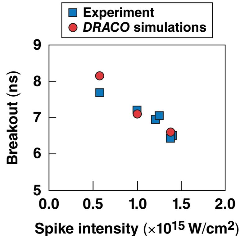
The agreement of measured and simulated shock-breakout times is better than 6%.
