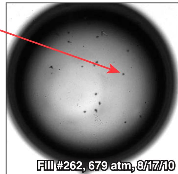
**Features do not continue to grow once the capsule is in the moving cryostat.**
