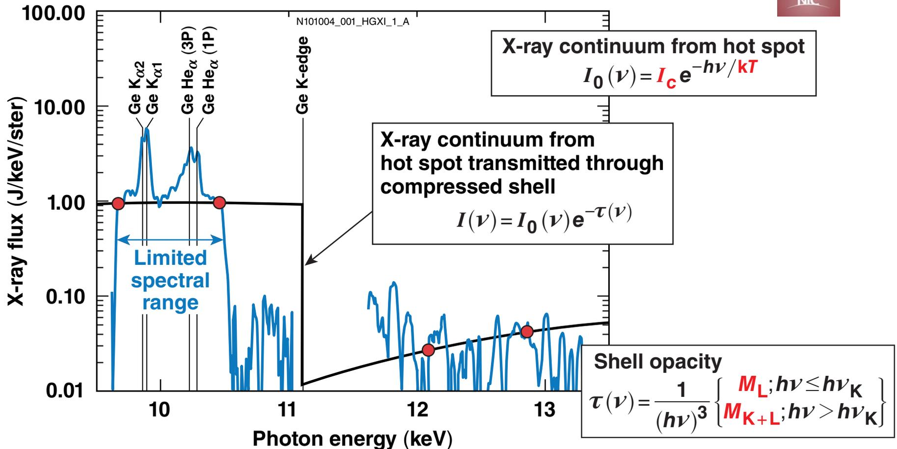
$T_e = 3 \pm 0.5$  keV is inferred from the slope of the x-ray continuum from the hot spot.
