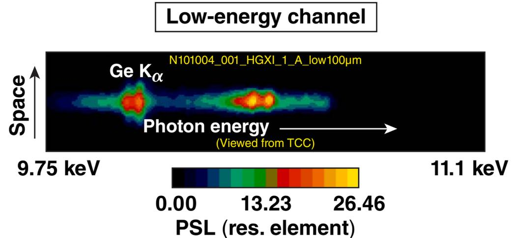
Spectral imaging discriminates implosion emission from hohlraum plasma emission.
