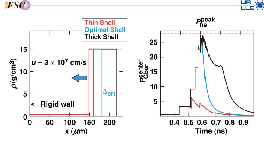
For  $\Delta > \Delta_{crt}$ , the shell kinetic energy poorly couples to the hot spot.
