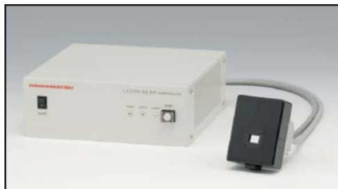
Hamamatsu LCOS-SLM Area: 12 \times 16 \text{ mm}^2 Resolution: 600 \times 792 ( 20\text{-}\mu\text{m} pixel) Dynamic range: 2 waves
