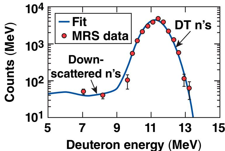
The MRS down-scatter fraction ( $\#n'/\#n$ ) is used to infer a fuel  $\langle \rho R \rangle_n$  of  $180 \pm 35 \text{ mg/cm}^2$
