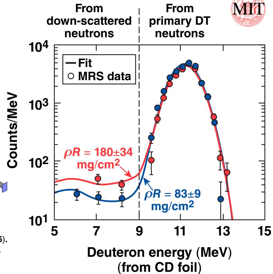
The MRS has been used on ~17 cryogenic DT implosions and measured areal densities from <100 mg/cm<sup>2</sup> to ~300 mg/cm<sup>2</sup>.
