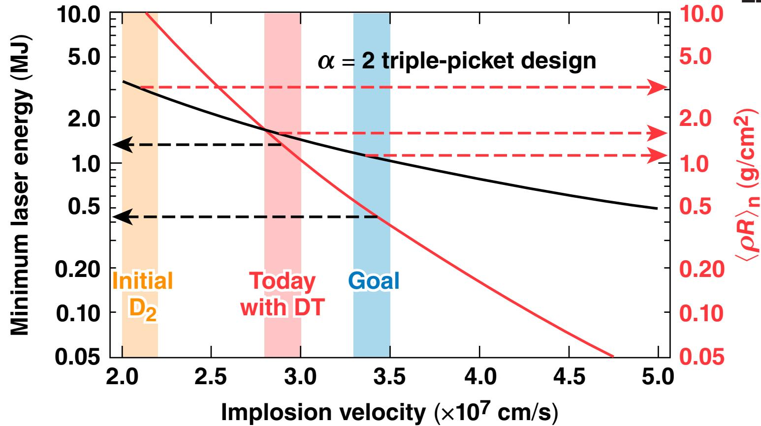
A  $V_{\text{imp}} \sim 3.5 \times 10^7$  cm/s is probably the OMEGA limit given intrinsic drive/ice nonuniformities.
