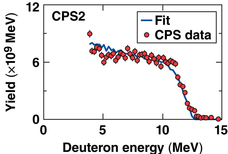
The spectrum is fully saturated indicating a  $\langle \rho R \rangle_n \gtrsim 180 \text{ mg/cm}^2$
