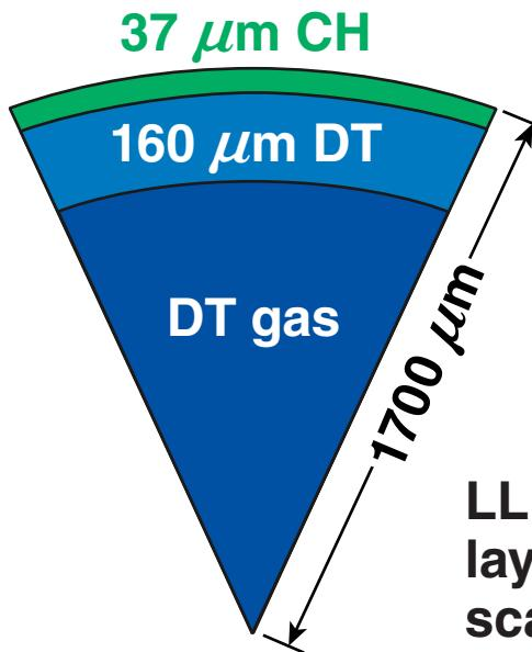
LLE has filled and layered an ignition-scale target with D<sub>2</sub>
