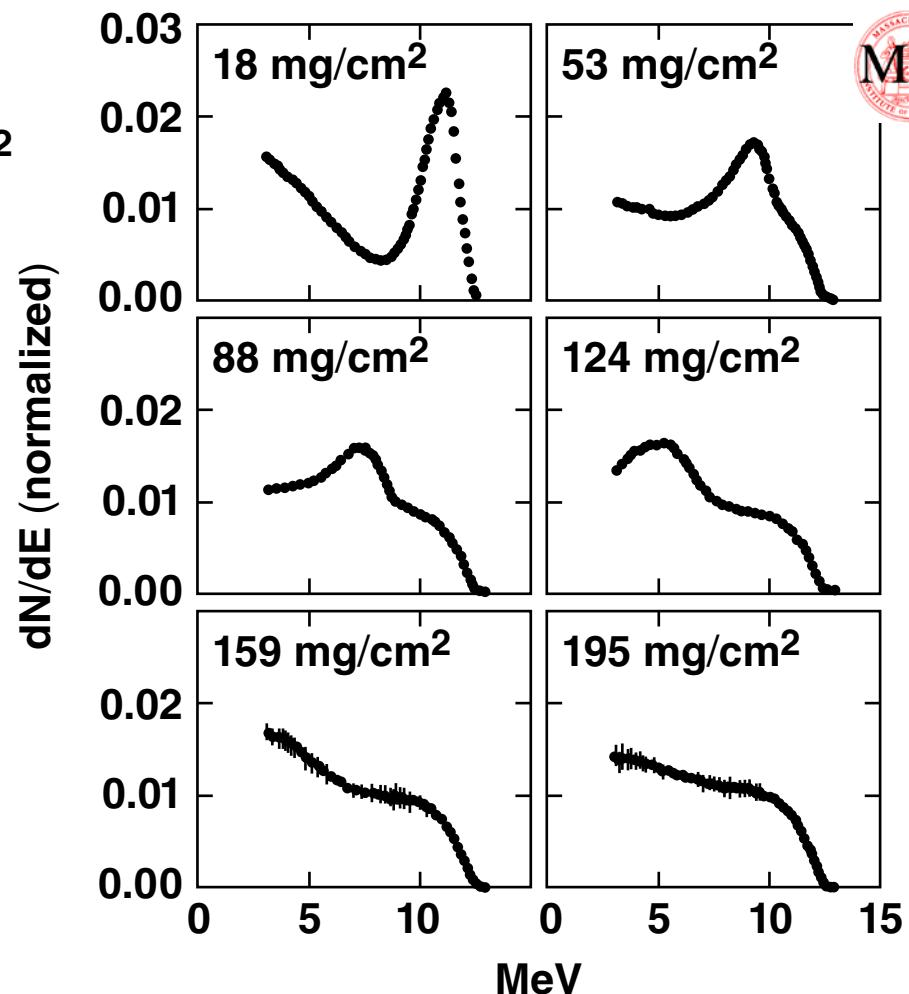
The shape of the KO-D spectrum no longer changes for  $\rho R > 180 \text{ mg/cm}^2$ .
