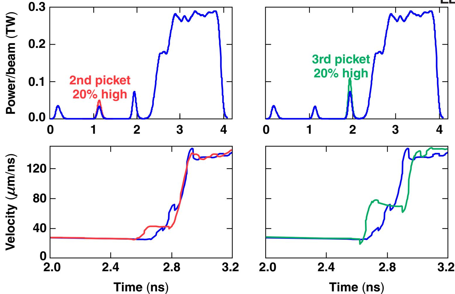
Shock coalescence can be measured more accurately using ASBO and SOP than the 100 ps requirement.
