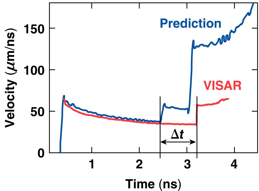
The delay in shock coalescence appears to be correlated with the energy of the first picket.
