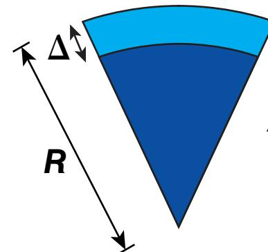
$$A_{\text{in}} = \frac{R}{\Delta} \approx 60 \left( \frac{V_{\text{imp}}}{3 \times 10^7} \right)^2 \left( \frac{p_{\text{Mbar}}}{100} \right)^{-2/5} \alpha^{-3/5}$$
