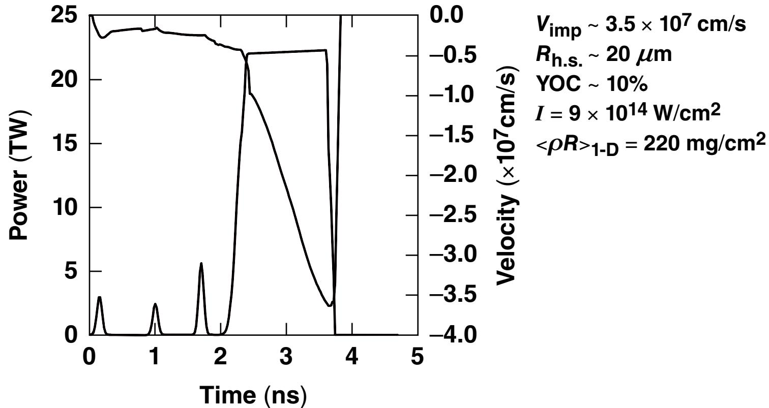
A higher-adiabat square main pulse is used to enhance shell stability.
