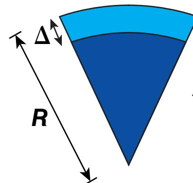
$$A_{in} = \frac{R}{\Delta} \approx 60 \left( \frac{V_{imp}}{3 \times 10^7} \right)^2 \left( \frac{p_{Mbar}}{100} \right)^{-2/5} \alpha^{-3/5}$$
