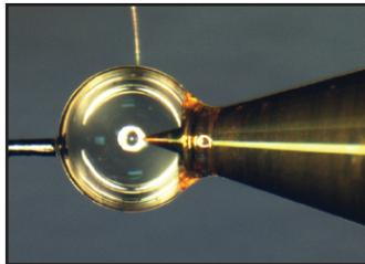
**Fill-tube-based FI cone-in-shell target**
