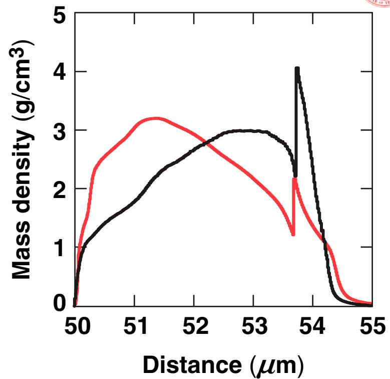
Adiabat is steeper inside the shell in triple-picket design
