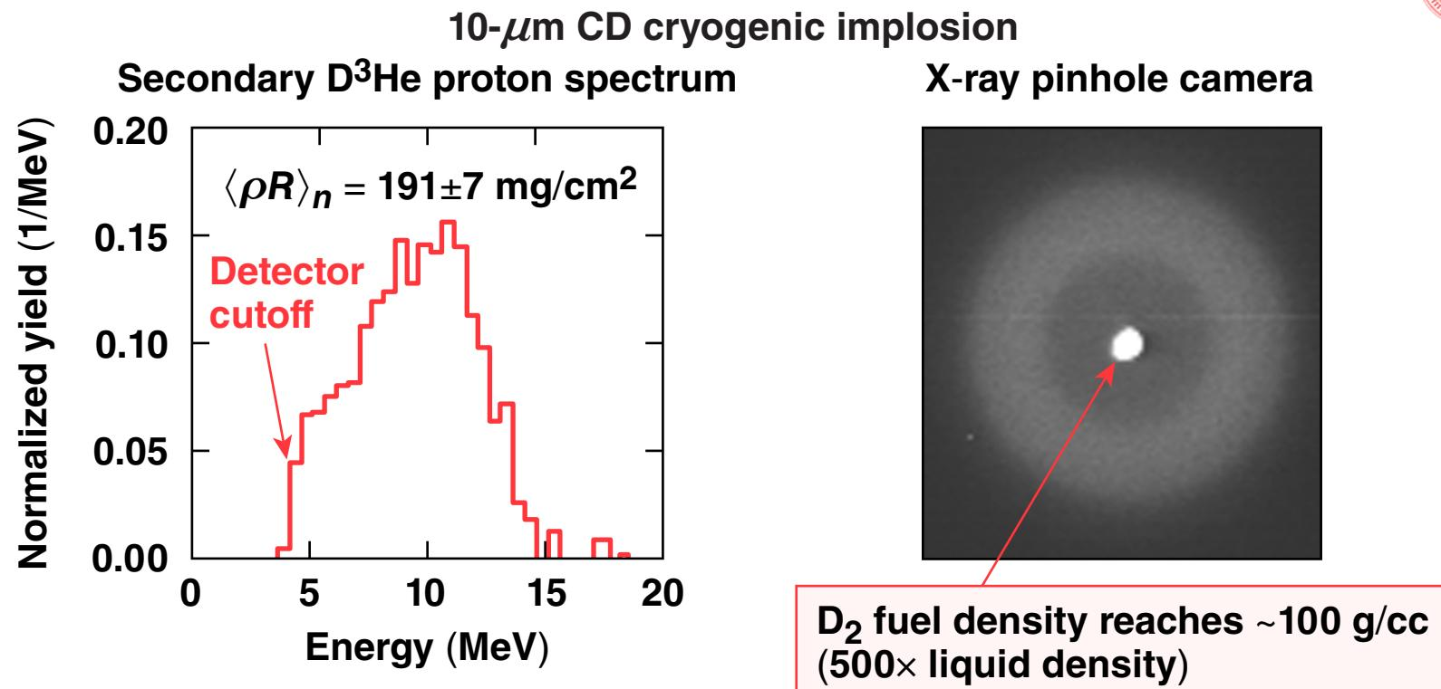
These are, by far, the highest areal densities measured in ignition-relevant laboratory implosions—very important for direct- and indirect-drive ignition.
