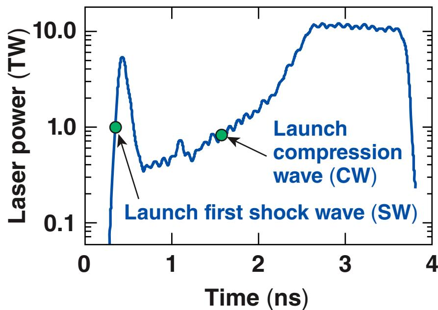
CW and SW must coalesce near the inner edge of the shell
