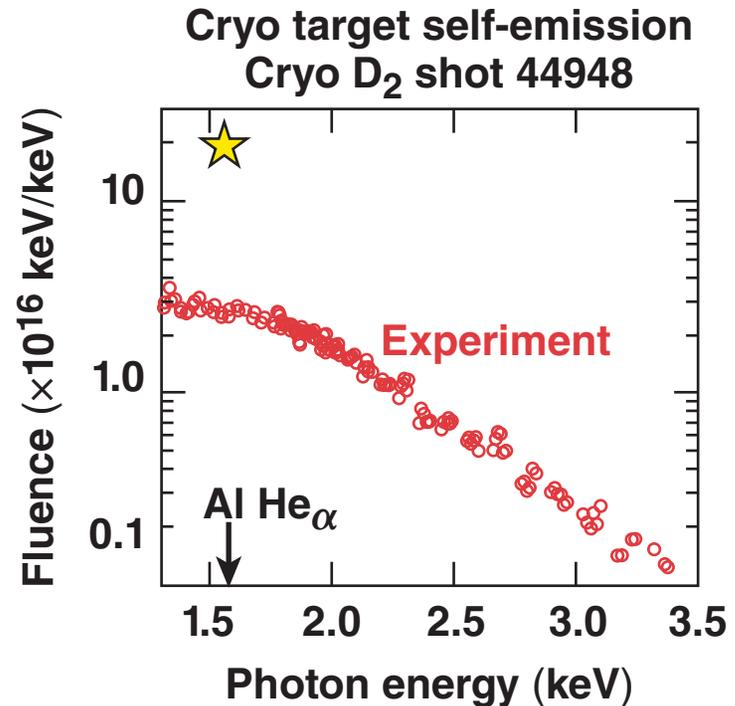
The OMEGA EP-generated Al emission is bright enough to backlight cryogenic targets.
