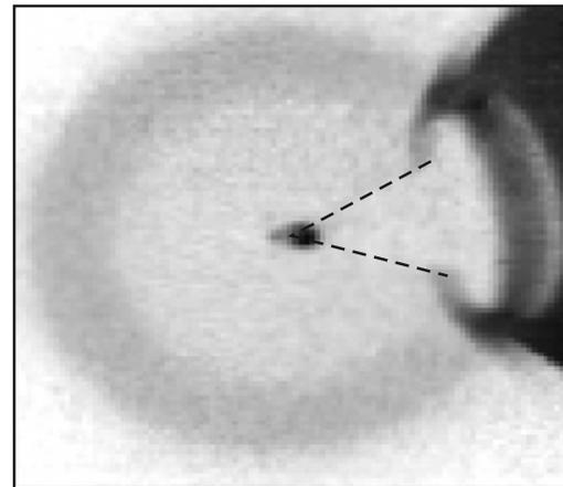
The hard x-rays produced by the short pulse interaction saturate the current neutron detectors.
