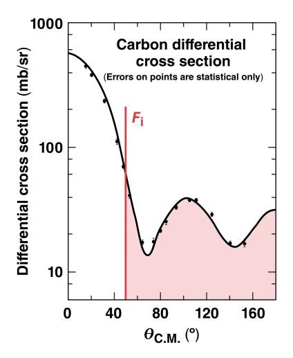
*F*<sub>n</sub> (the fraction of incident neutrons) can be calculated based on the total scattering cross section.
