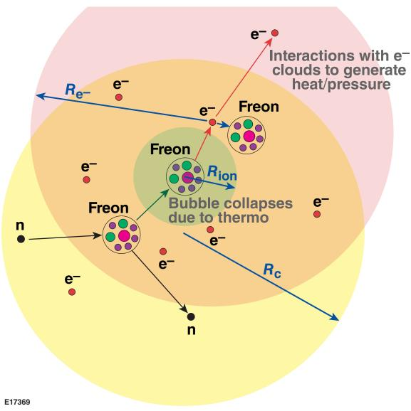
Since the recoil-ion range is short, energy must be deposited in a volume ~R<sub>c</sub><sup>3</sup> by energetic (several hundred eV) electrons.
