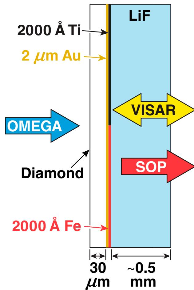
**LiF remains transparent at pressures less than 6 Mbar.**
