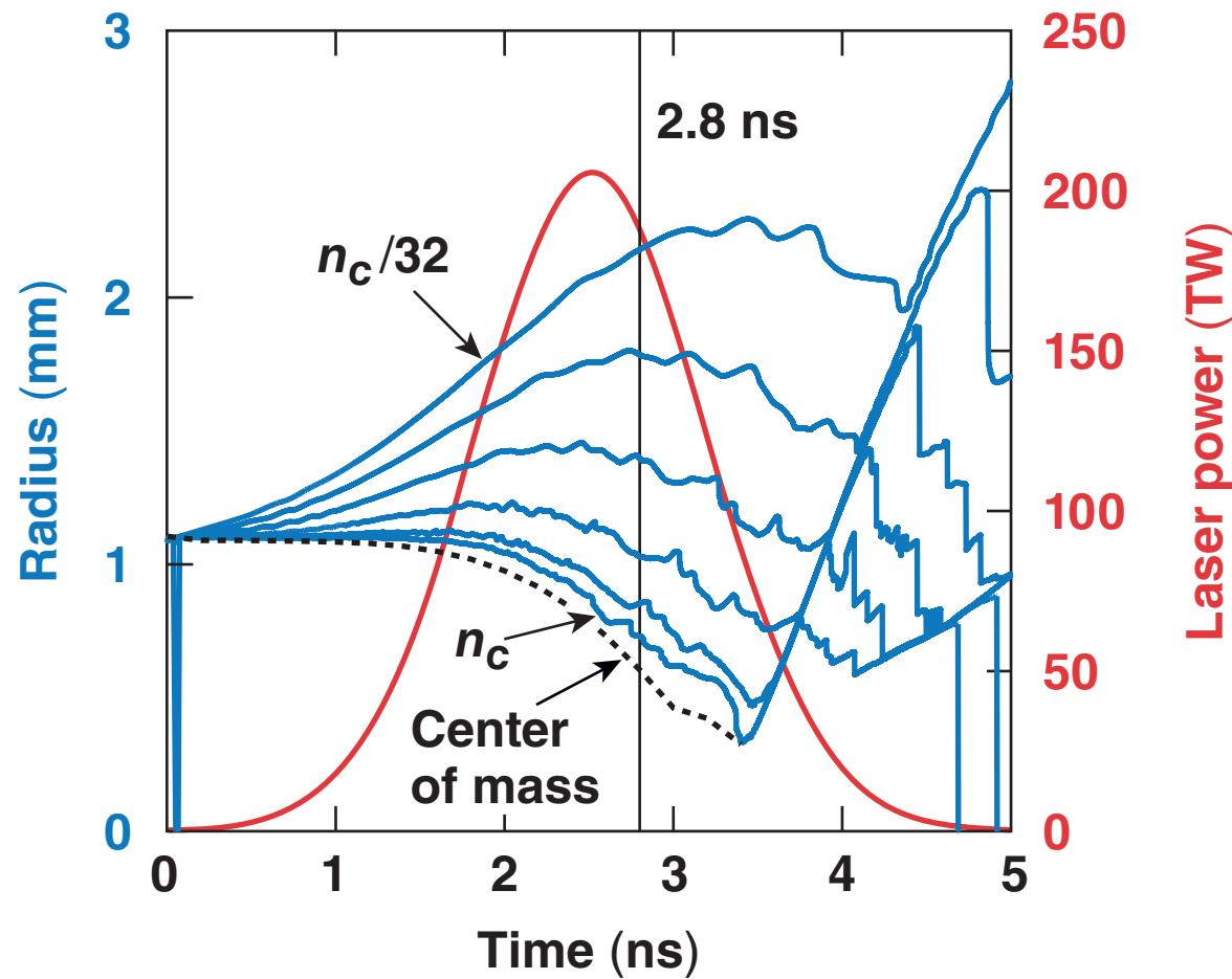
**At 2.8 ns the center-of-mass radius is  $600 \pm 6.5 \mu\text{m}$
