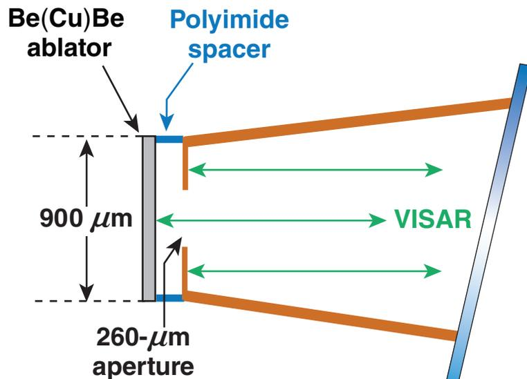
Window test at  $T_{\text{rad}} = 180 \text{ eV}$  without  $\text{D}_2$
