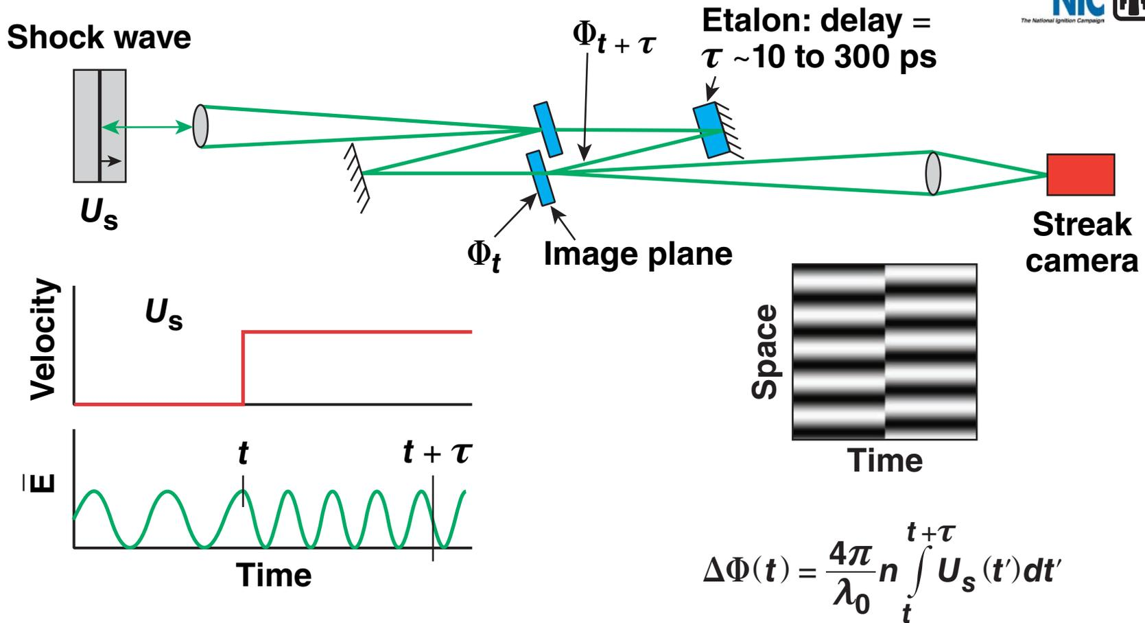
VISAR has time resolution  $<30$  ps and a velocity precision of  $\sim 1\%$ .
