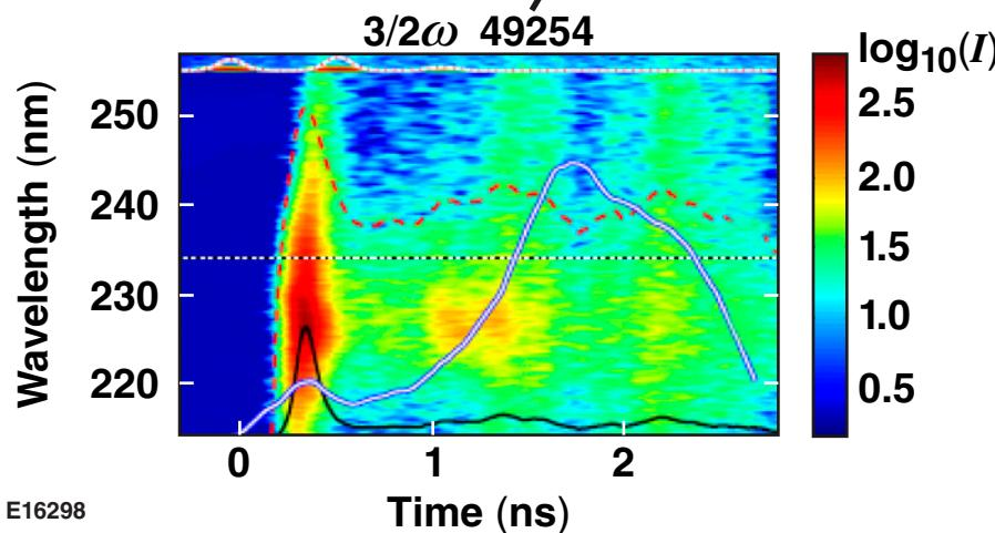
Only a single burst of x rays is observed from vacuum hohlraums because they do not have an LEH window
