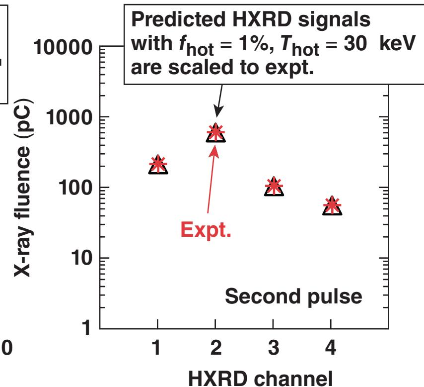
**$f_{\text{hot}}$  and  $T_{\text{hot}}$  can be estimated from HXRD signals**
