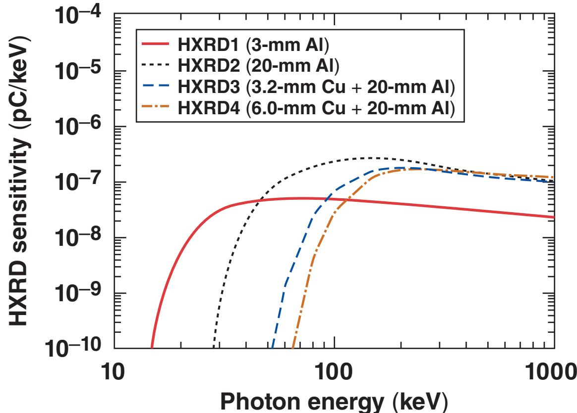
Relative calibration → filter transmission × scintillator absorption
