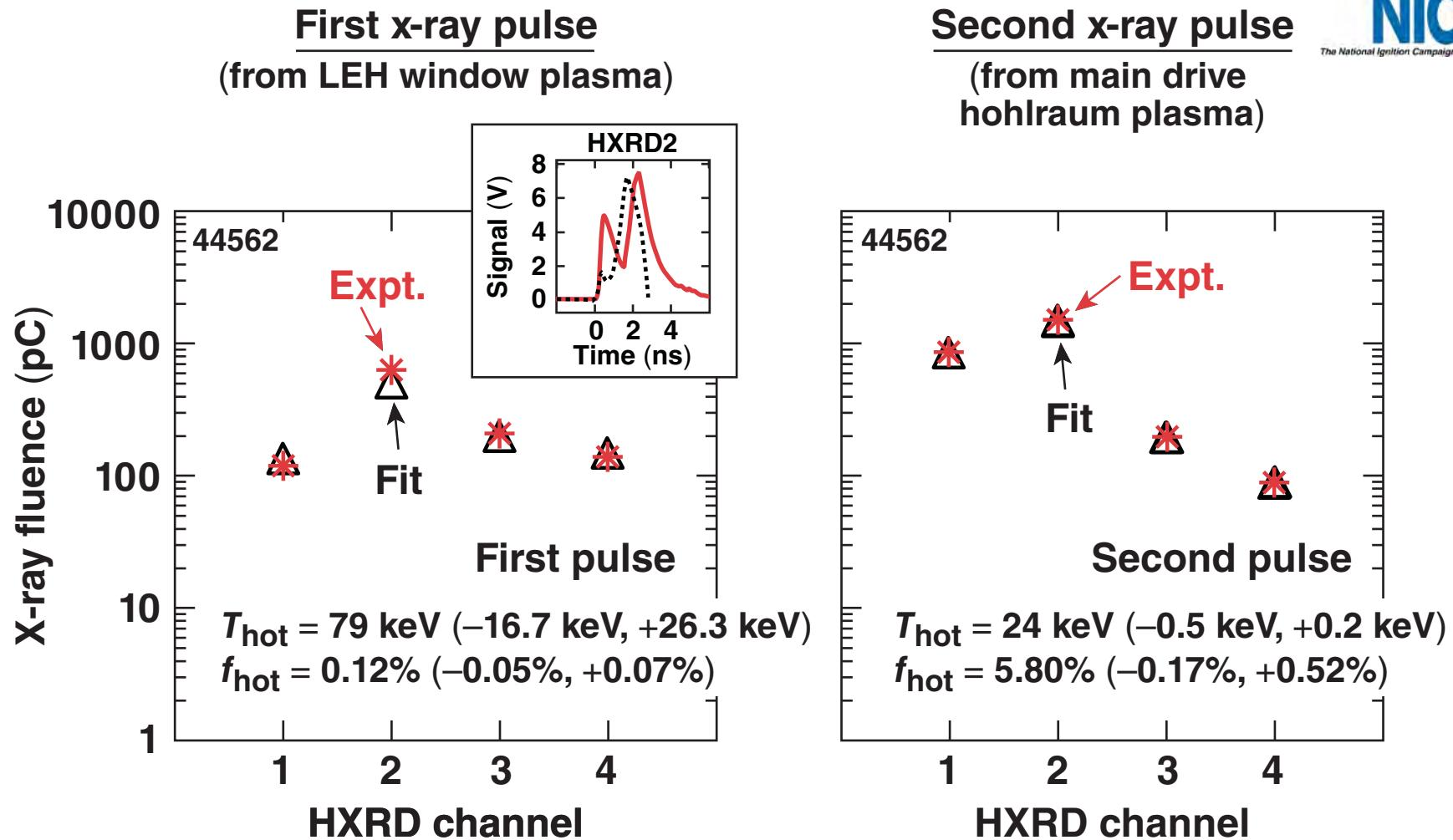
HXRD signals are sensitive to changes in  $f_{\text{hot}}$  and  $T_{\text{hot}}$
