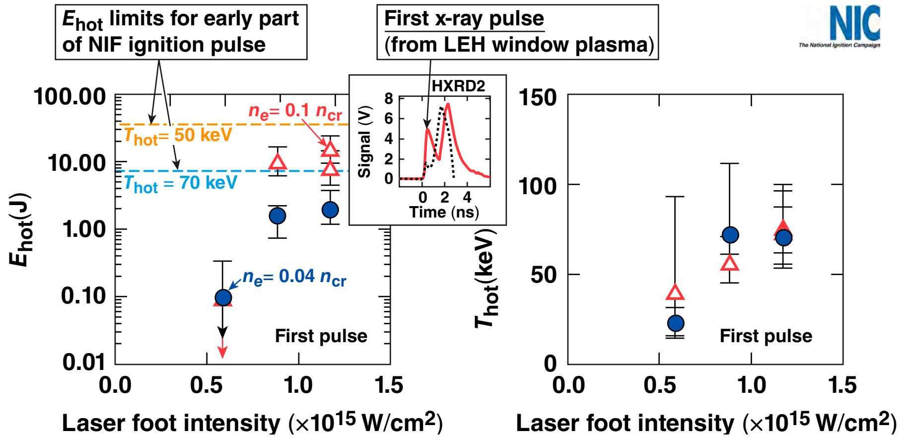
$E_{\text{hot}}$  and  $T_{\text{hot}}$  drop rapidly below this threshold
