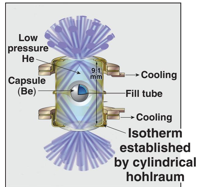
Low-mode thermal symmetry must be actively controlled in a hohlraum
