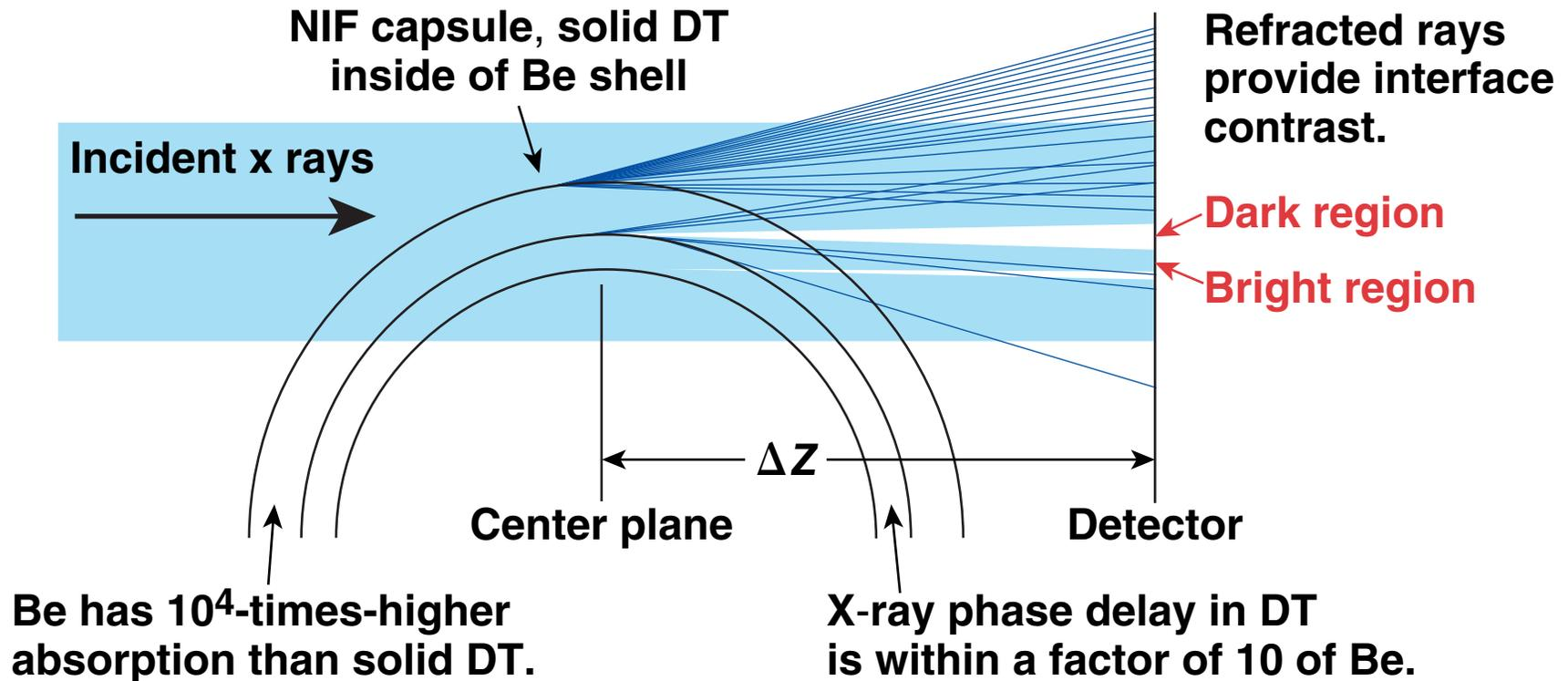
Need sufficient spatial coherence (plane wave or point source) to obtain good contrast for a given imaging configuration.
