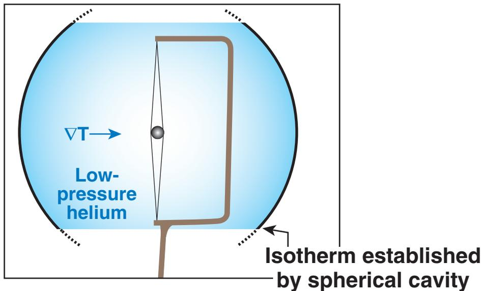
IR illumination imposes low-mode asymmetry by preferentially heating the target structures
