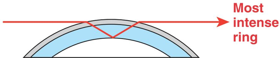
Light reflected off the inner surface creates a bright ring in a backlit image.
