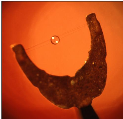
3 to 7- $\mu\text{m}$  SiO<sub>2</sub> shells with 5- $\mu\text{m}$ -thick DT layer
