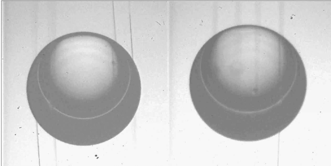
**“Single-crystal” ice layers grown at the triple point require temperature control to mK precision**
