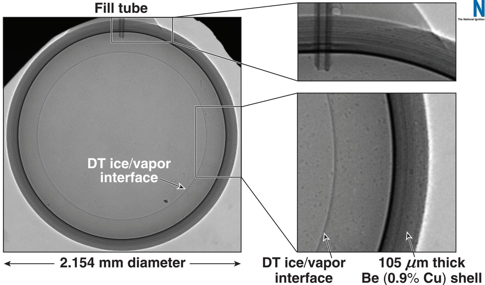
The surface ring is analyzed for the Fourier components using a process similar to that used with shadowgraphy.
