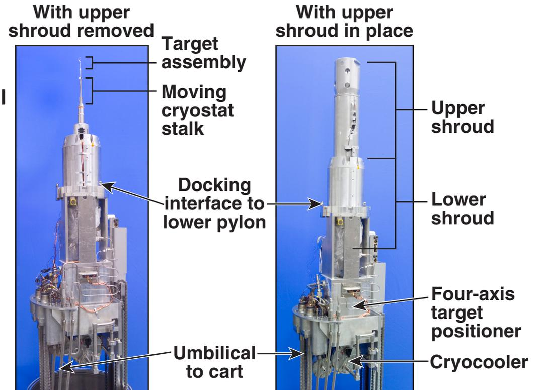
Cryostat assembly is for target positioning and life support.
