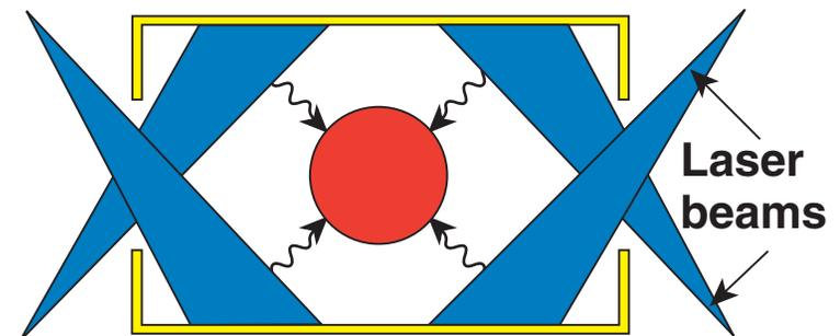
Hohlraum using a cylindrical high-Z case
