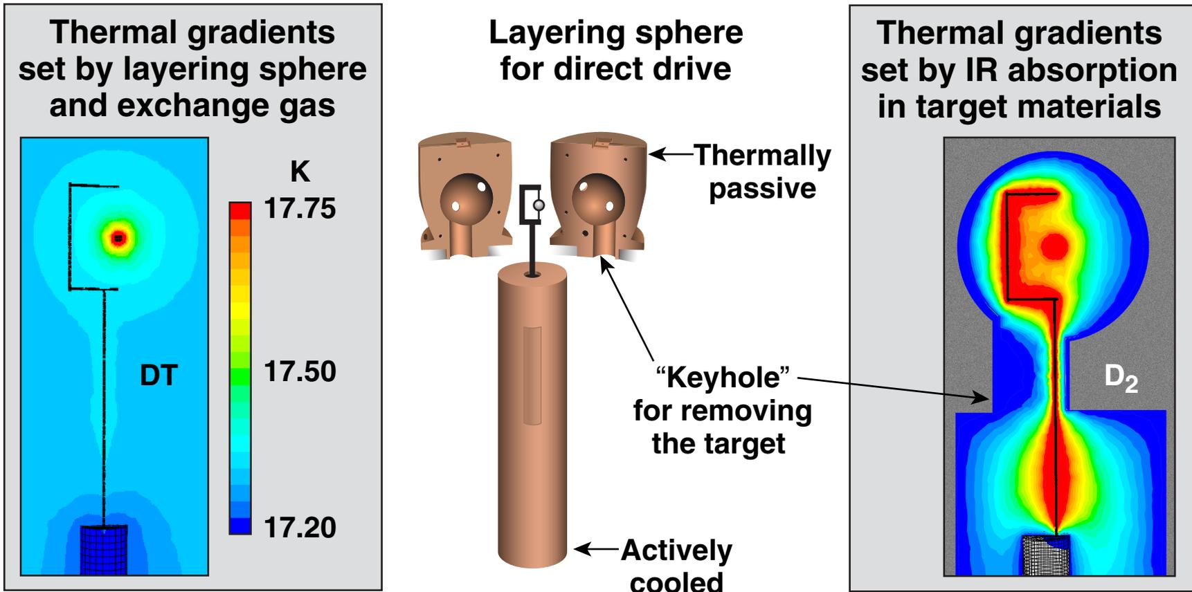
For direct-drive targets, thermal symmetry is achieved with clever design rather than active controls
