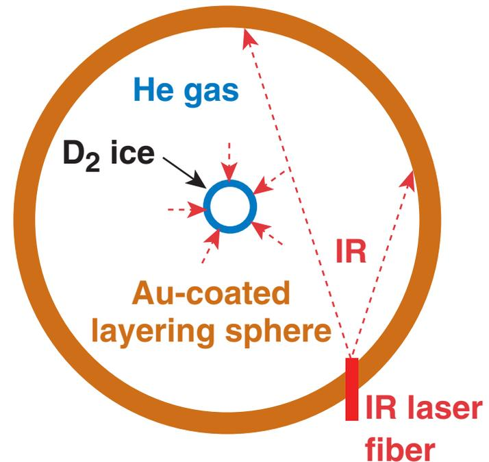
For IR-layering,<sup>2</sup> infrared light ( $\lambda \sim 3 \mu\text{m}$ ) preferentially deposits heat into the bulk D<sub>2</sub> (or DT) ice
