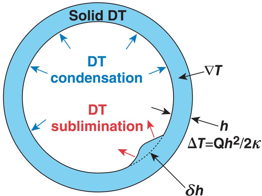
For  $\beta$ -layering,<sup>1</sup> the recoil  $e^-$  from the radioactive decay of the tritium deposits heat into the bulk DT ice
