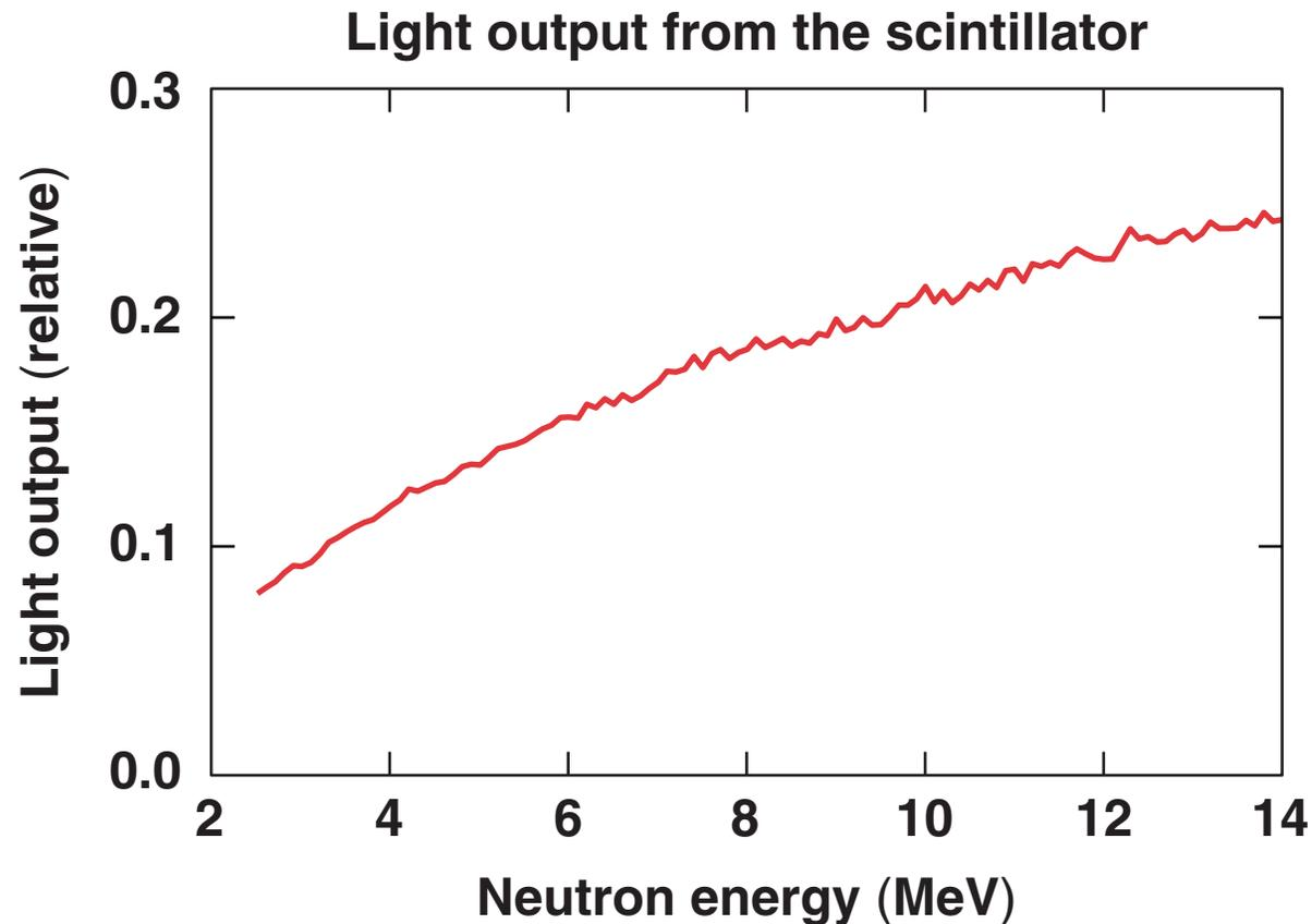
Monte Carlo model\* calculates light output from  $2 \times 2$ -cm BC-422 scintillator.
