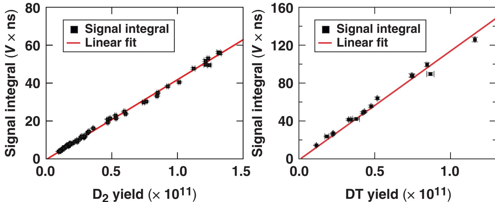
Both  $D_2$  and DT neutron calibrations have an accuracy of 10%.
