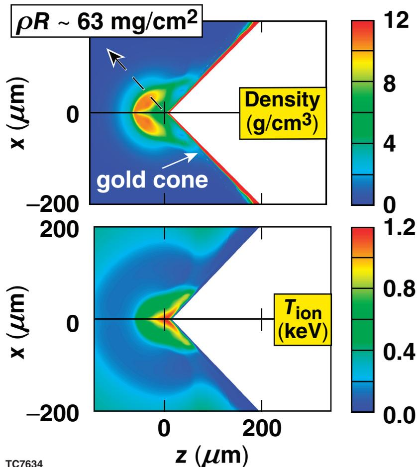
Experiment: 24- $\mu\text{m}$  CH, 22 kJ in 1-ns square, peak compression
