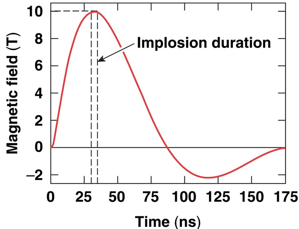
Magnetic field at the center of the coils calculated for a 100-nF capacitor and 4-mm-diam Helmholtz coils
