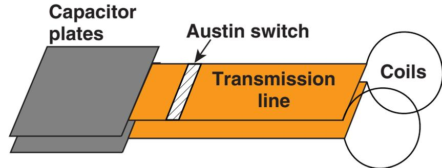
Experimental setup of Helmholtz coils and capacitor
