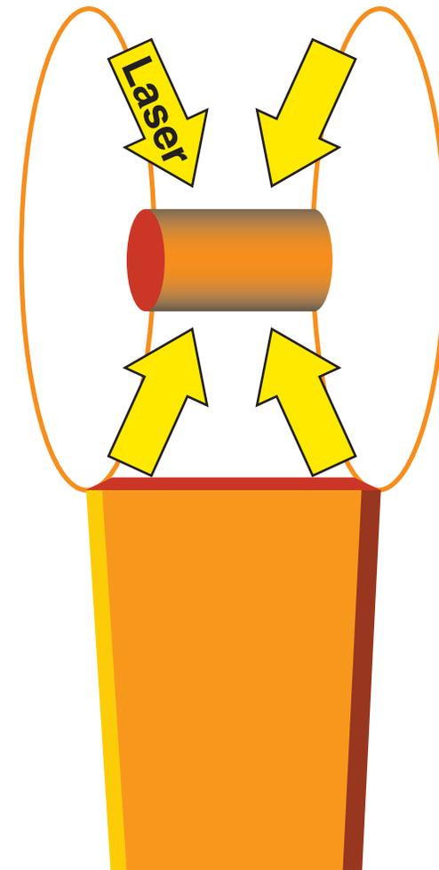
**Helmholtz coils and implosion target.**
