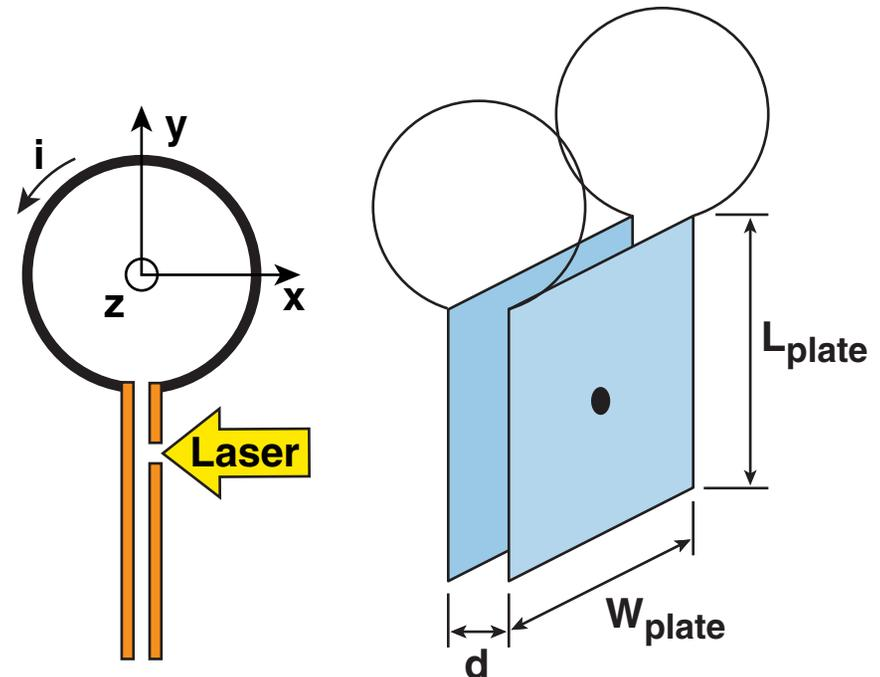
Helmholtz coils connecting the two capacitor plates in laser-driven setup
