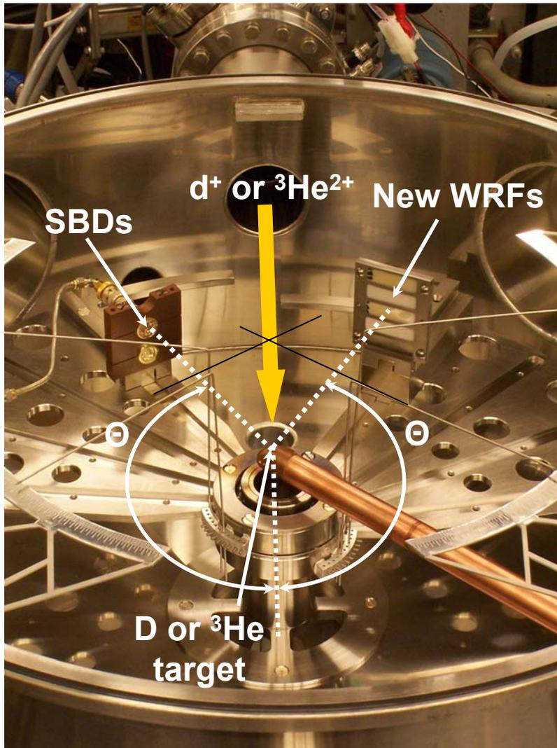
**D<sup>3</sup>He-protons (or DD-protons) produced at same angle ( $\Theta$ ) have same energy. These fusion products of same energy can be simultaneously monitored by several calibrated SBDs and new ICF diagnostics to be tested or calibrated. In this particular case new WRFs are being calibrated.**
