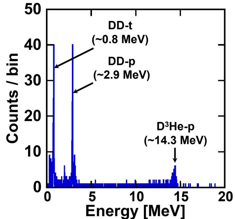
The accelerator also produces DD-neutrons, which will be used for developing and optimizing several types of ICF diagnostics
