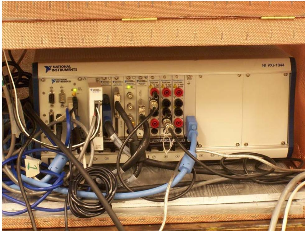
**A National Instruments PXI system is being implemented to replace many of the older control elements, and add new diagnostic functionality and expandability.**
