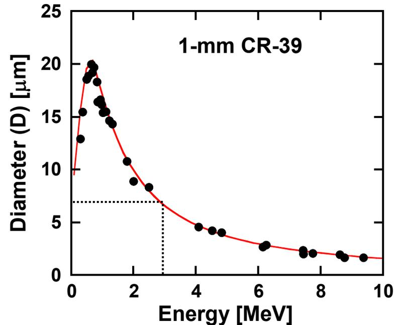
A calibrated mapping between track diameter and proton energy can be obtained, since track diameter is proportional to  $dE/dx$ .
