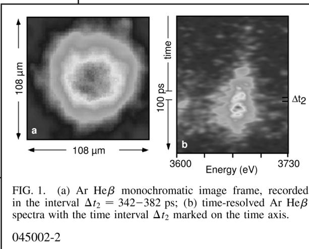
FIG. 1. (a) Ar He $\beta$  monochromatic image frame, recorded in the interval  $\Delta t_2 = 342\text{--}382$  ps; (b) time-resolved Ar He $\beta$  spectra with the time interval  $\Delta t_2$  marked on the time axis.
