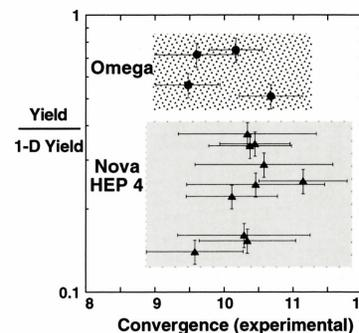
FIG. 4. Comparison of measured yield normalized to calculated 1D clean yield vs measured convergence ratio for implosions driven by single ring per side Nova (triangles) vs multiple ring per side Omega (circles) hohlraums.
