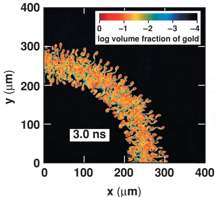
*RAGE* simulation of the volume fraction of a gold marker in a direct-drive cylindrical mix implosion
