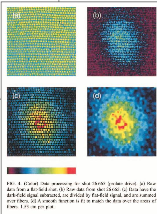
FIG. 4. (Color) Data processing for shot 26 665 (prolate drive). (a) Raw data from a flat-field shot. (b) Raw data from shot 26 665. (c) Data have the dark-field signal subtracted, are divided by flat-field signal, and are summed over fibers. (d) A smooth function is fit to match the data over the areas of fibers. 1.53 cm per plot.
