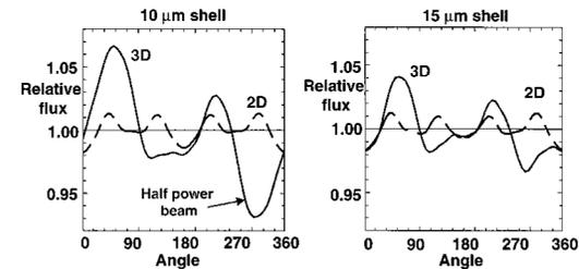
FIG. 12. View factor simulations using the actual power in each of the 42 beams that went into the hohlraum for shots 19082 (left) and 19083 (right). The 2D dashed curves were made by azimuthally averaging each laser beam.
