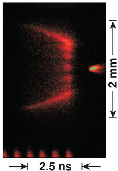
Imaging x-ray streak camera image of cylindrical implosion. Spikes of an imposed  $m = 14$  perturbation burnthrough just before the end of the 2.5-ns drive pulse.
