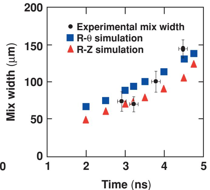
Comparison of experimental measurements of mix width in time with *RAGE* simulation
