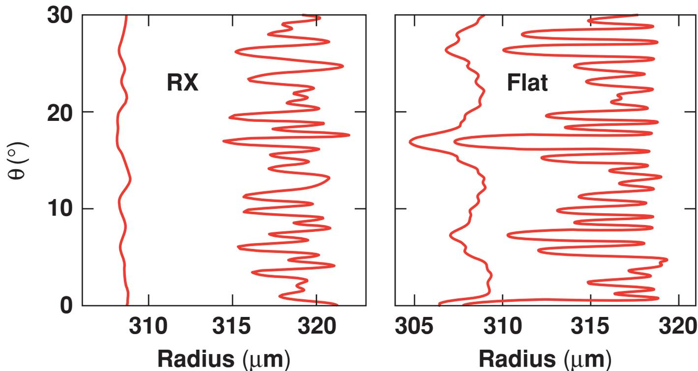
**RX:**  $\sigma_{\text{rms}}(\text{outer}) = 1.73 \mu\text{m}$     **Flat  $\alpha = 3$ :**  $\sigma_{\text{rms}}(\text{outer}) = 2.90 \mu\text{m}$
