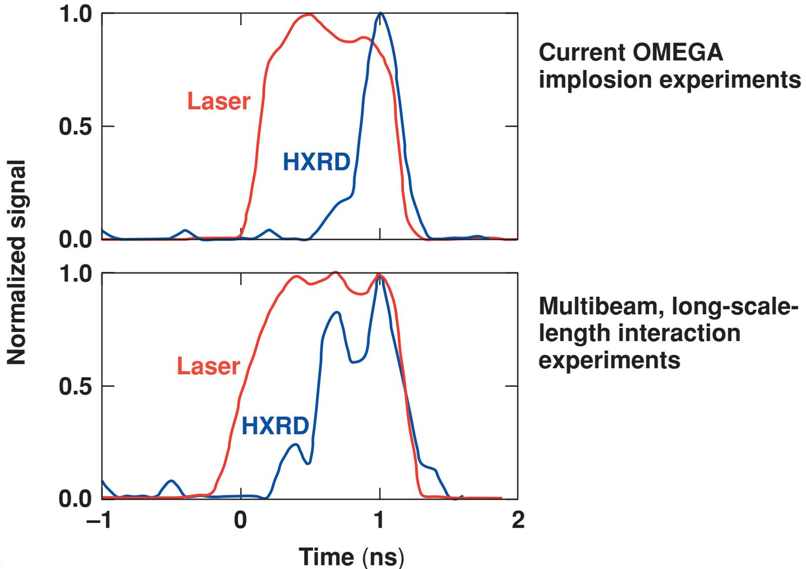
The hard-x-ray ( $> 50\text{-keV}$ ) signal depends only on the overlapped intensity and saturates above  $10^{15} \text{ W/cm}^2$
