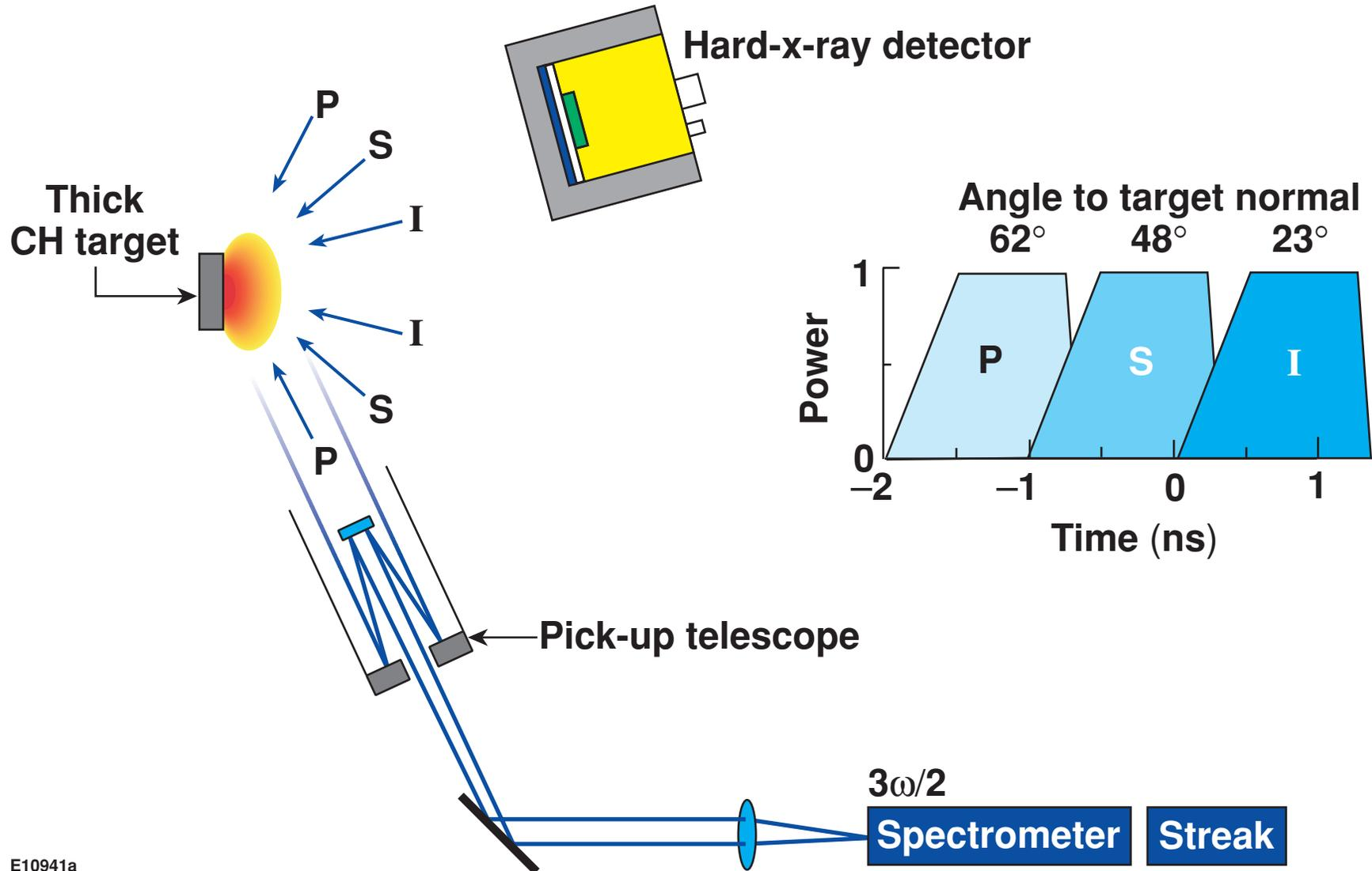
For current OMEGA implosions the temporal evolution of the hard x rays reflects the increasing density scale length
