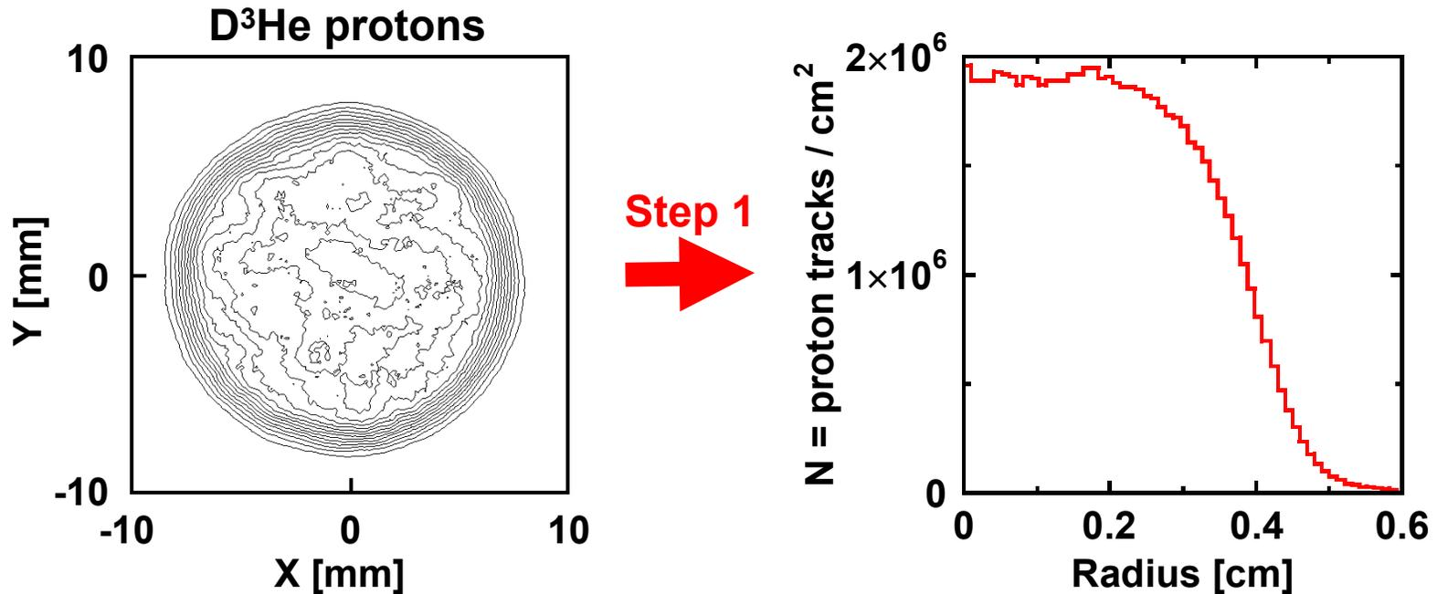
**Step 1:** Calculate the proton hit density ( $N$ ) as a function of radius in the image plane.
